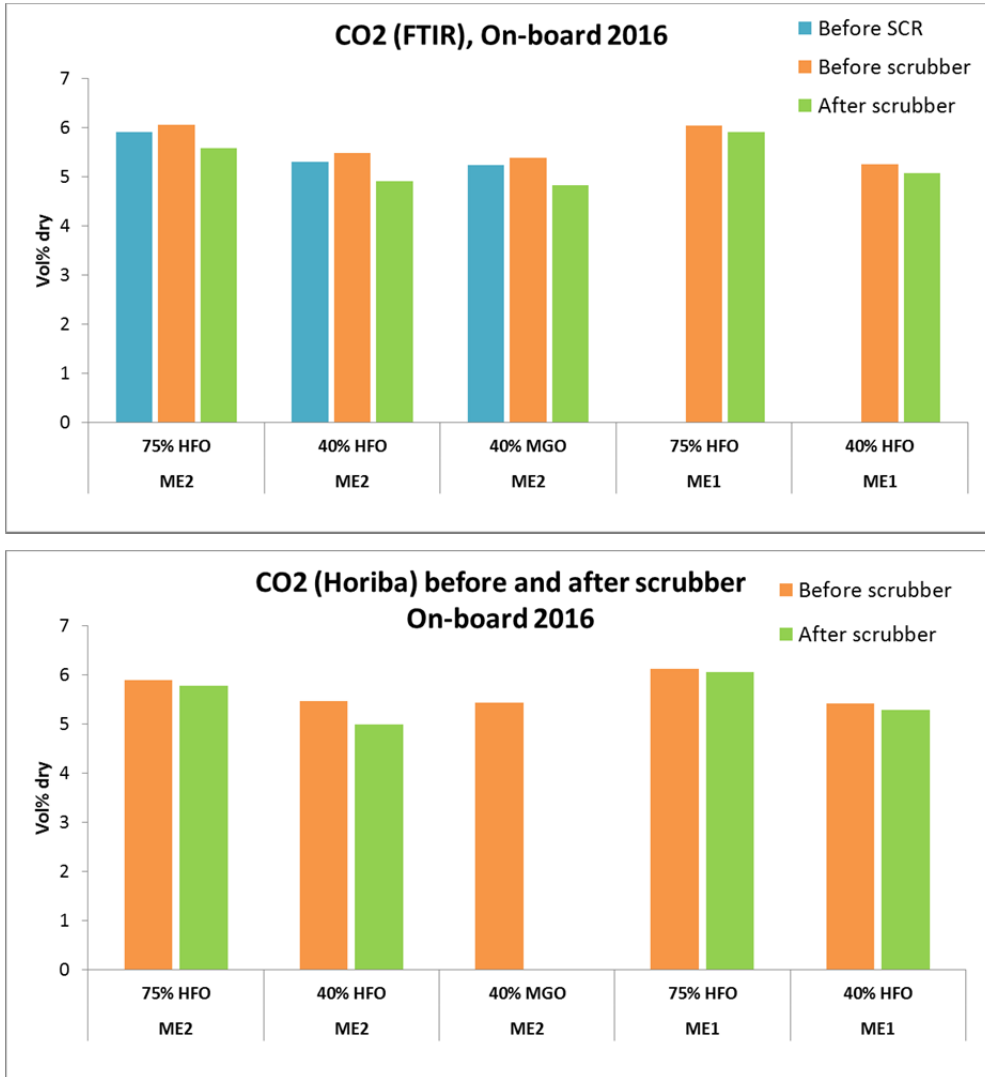
Figure 3.1. CO 2 concentrations measured with the FTIR (above) and Horiba (below) before and after the scrubber.
