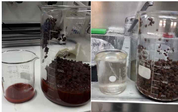
Figure 5. Leca® materials treated with \text{Fe}(\text{NO}_3)_3 then oven dried were washed with deionised water (left) until the leachate was visually clear (right).
