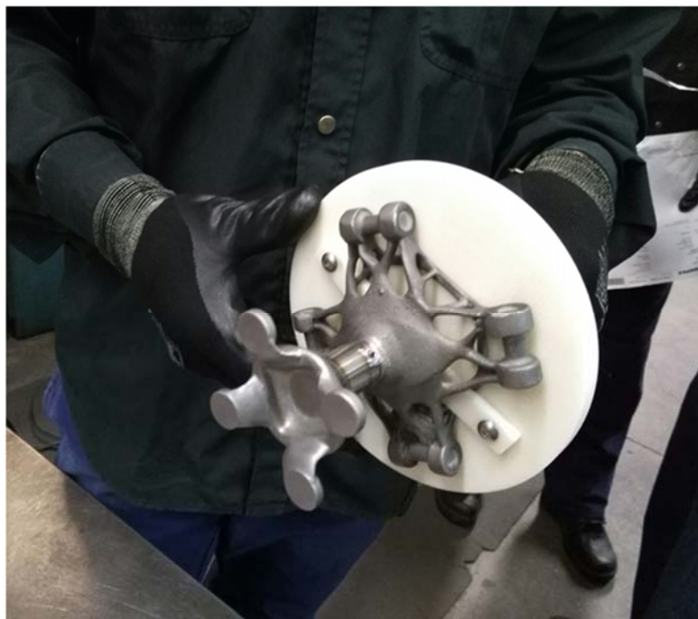
Figure 19. The blade hub after laser welding.
