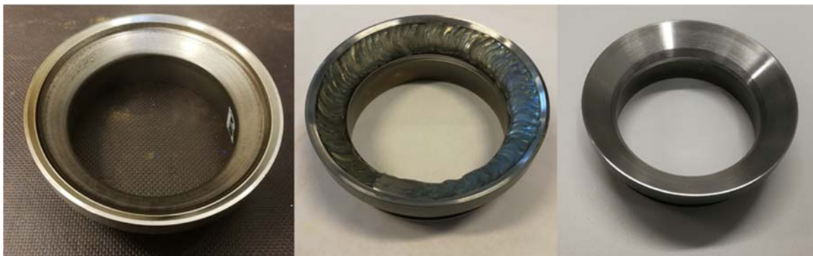
Figure 12. From Left to right: The original seat ring, the pieces after directed energy deposition, and the finished piece.
