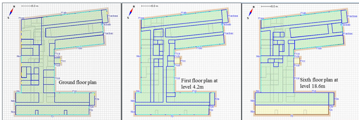
Figure 3 Typical ground floor plan, first-floor plan at level 4.2m, and sixth-floor plan at level 18.6m with thermal zones as described in Table S2, modeled in IDA ICE.
