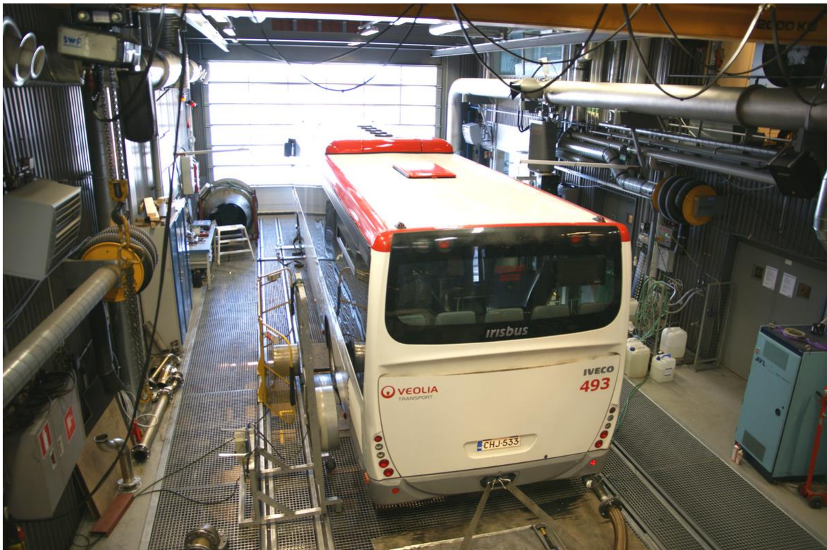
Figure 2. A view of the test facility. The CVS dilution tunnel can be seen in the upper right-hand corner.
