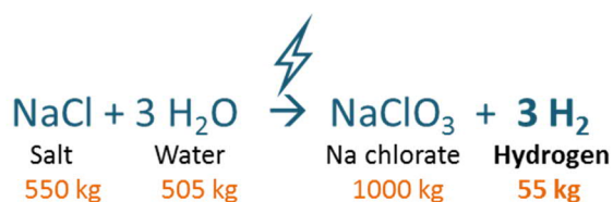
Figure 22. Overall reaction for an ideal chlorate plant.
