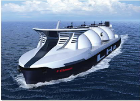
Figure 35. Conceptual design of a 160 000 m 3 liquid hydrogen carrier. (Kamiya et al. 2015)
