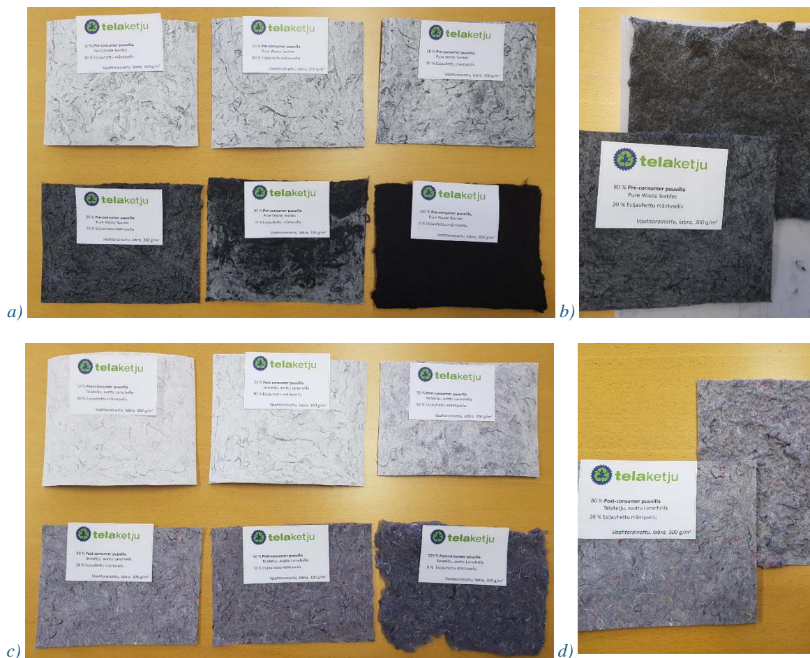
Figure 38 Foam laid samples produced in lab: a) pre-consumer cotton (from Pure Waste Textiles) in mixtures with pulp: R-CO content 10 %, 20 %, 50 %, 80 %, 90 % and 100 %; b) difference between wire side and upper side of 80 % R-CO containing sample; c) & d) corresponding samples than in a) & b) but produced using post-consumer R-CO fibres from Laroche opening trials
