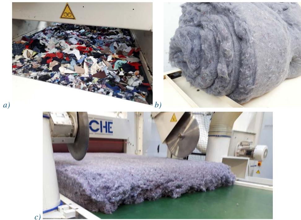
Figure 34 a) Sorted fabrics cut to pieces in two directions at Laroche; b) opened fibres; and c) air-laid felt from recycled material suitable e.g. for isolating purposes
