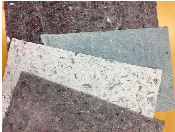
Figure 43 Textile fibre sheets made of post-consumer cotton, polyester (PET) and fibre dust
