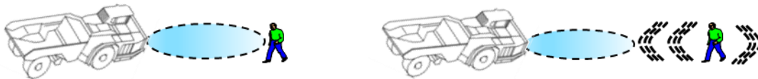
Figure 42. Left: On-board safety system on an autonomous mobile work machine. Right: Detector on each autonomous mobile work machine and active tags on each moving object. (Figure: dumper hauler 63 ).
