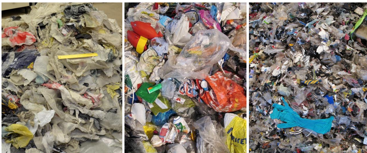
Figure 3. Plastic waste feedstocks used in thermolysis tests. LTW on the left, F-SUM in the middle and F-SRF on the right.
