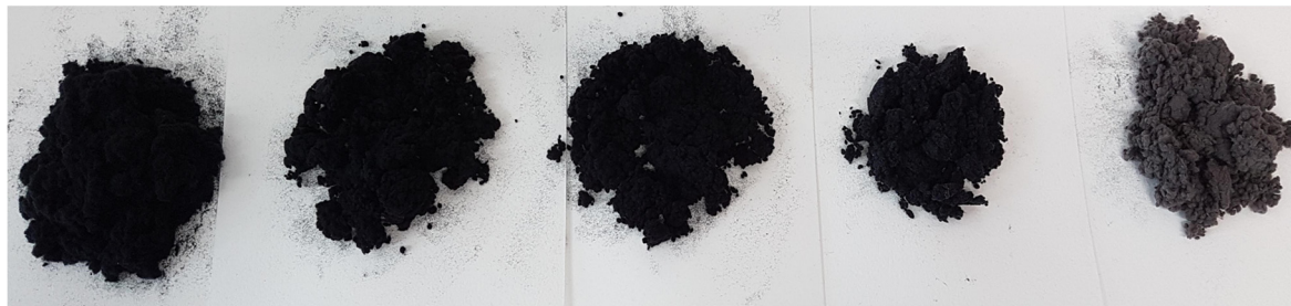
COpi3 shortened brightness 1.9 % SBP-1.3/60 brightness 1.9 % PF-1.3/60 brightness 2.5 % O 3 -1/RT brightness 3.4 % NaOH-40/80 brightness 15.8 %
