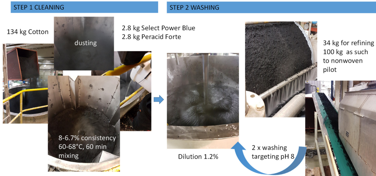
Figure 23 Cleaning pilot process at KCL
