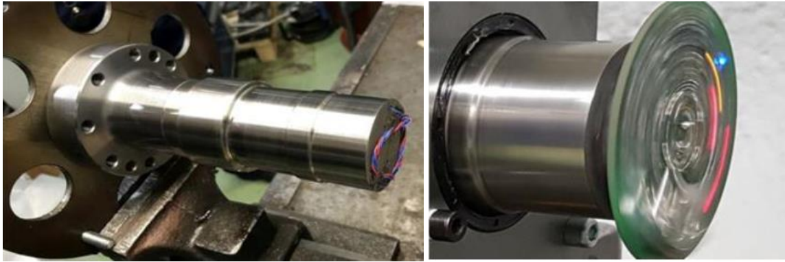
Figure 6. 3D printed metal smart shaft that has an accelerometer inside and wireless data transfer. © 2020 VTT Technical Research Centre of Finland Ltd.
