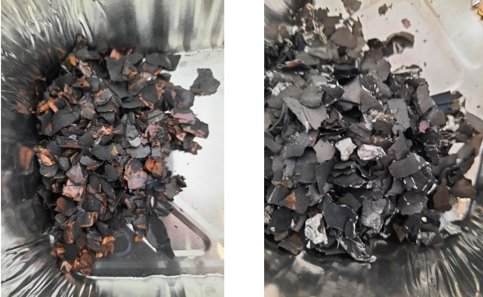
Figure 9: Impure Cu and Al foils, upon which active electrode materials still reside.
