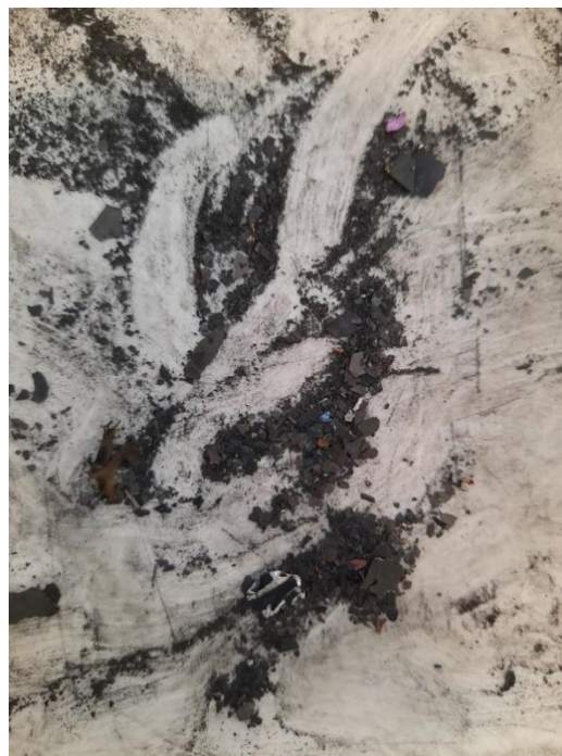
Figure 10: Further fines, composed of graphite, metal oxides and foils pieces, generated from the size class of 4-5.6 mm.
