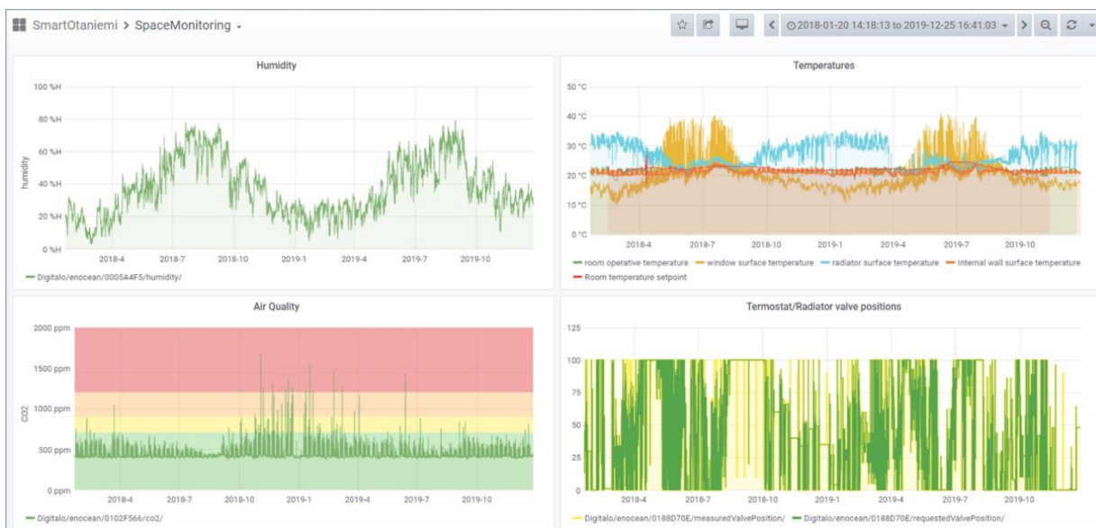
Figure 17. An example of the VTT research platform connected Grafana dashboard for monitoring space data (case Vuorimiehentie 3, Space A105, last two years of data).
