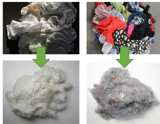
Figure 34 Effect on colour sorting on the colour of the mechanically opened fibres
