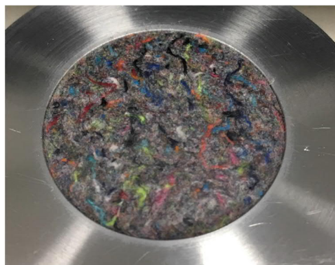
Figure 54 Bee wax coating on rags paper (discarded clothes) made merely of 65% PES, 35% CO after 30,000 rounds in Martindale test shows no wear and tear. Different colour fibres originate from discarded mixed fibre clothes. The texture of the paper is smooth and leather-like. Photo: Minna Cheung
