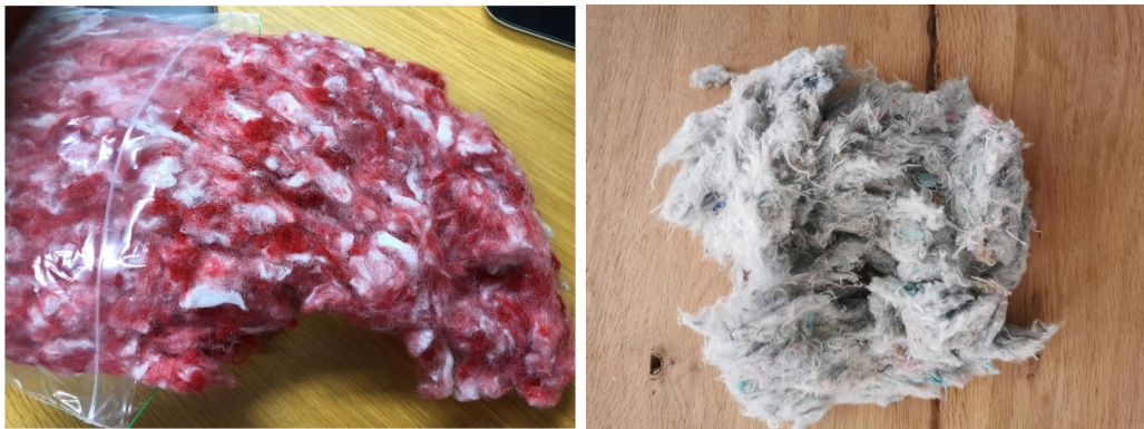
Figure 41 Opened fibres from a) technical PA warp knit from Mirka and b) woven PES/CO work-wear from Touchpoint
