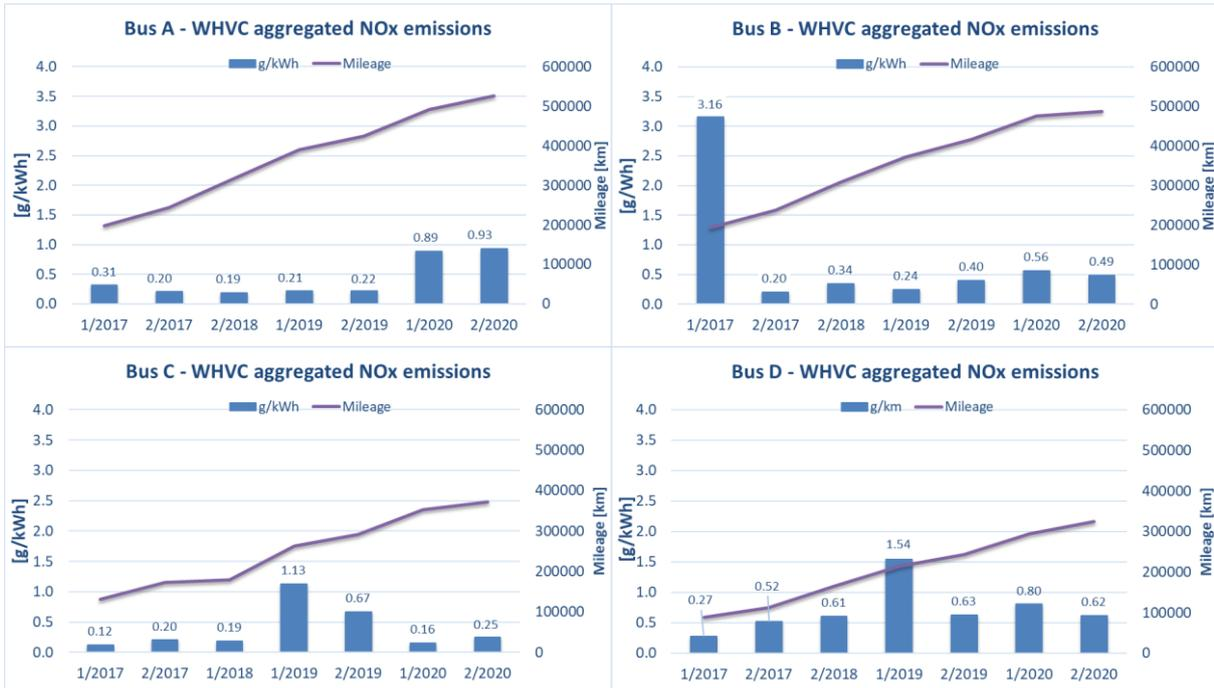
Figure 18: Aggregated (cold + hot cycle) NO<sub>x</sub> emissions on WHVC. Euro VI limit value on WHTC is 0.46 g/kWh.
