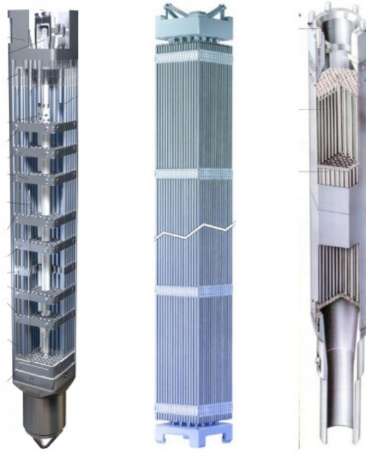
Figure 2-1. Fuel assemblies (not to scale) from Olkiluoto 1-2 (BWR) and Olkiluoto 3 (EPR/PWR) and Loviisa 1-2 (VVER-440) nuclear power plants units. Figure by Posiva (n.d.)Posiva.
