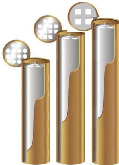
Figure 2-2. Illustration of copper canisters and cast-iron inserts for the spent fuel from Loviisa LO1-2 unit (left), Olkiluoto OL1-2 unit (middle) and from Olkiluoto OL3 unit (right). From Raiko (2013).
