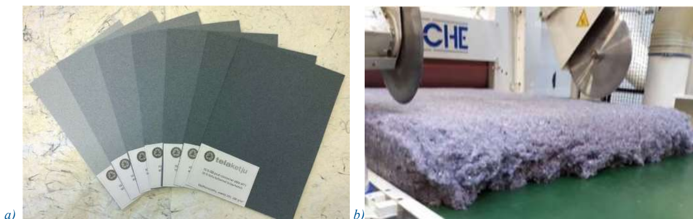
Figure 7 a) Thin foam formed sheets from very short cotton fibres (dust from the mechanical opening process of denim) mixed with pulp fibres. b) Thick air-laid felt from mechanically opened post-consumer fibres bonded with bi-component fibres. (Heikkilä et al. , 2019b).
