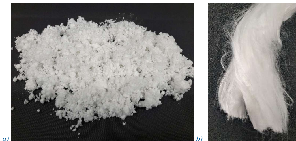
Figure 11 Separated PES fraction (a) and wet-spun Biocelsol fibres (b) from the dissolved cotton fraction (Vehviläinen et al. , 2018).
