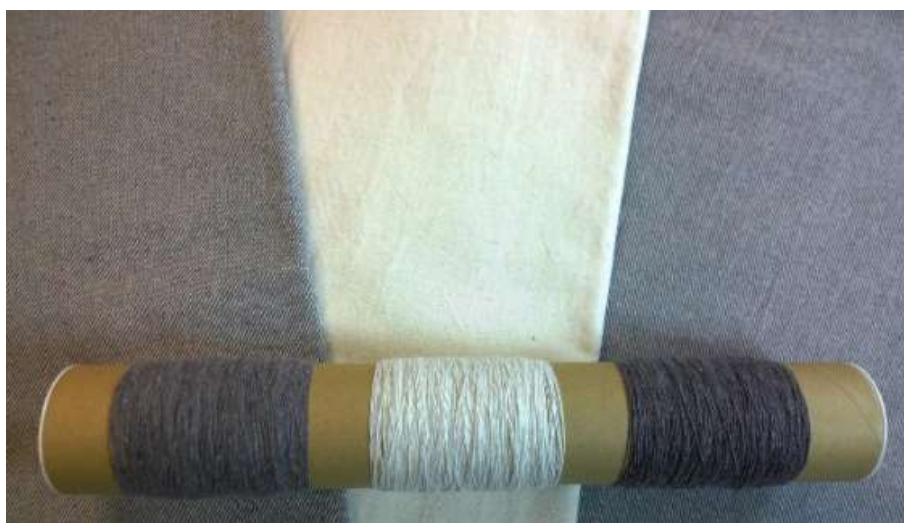
Figure 6 Yarns and woven fabrics made from mechanically opened fibres (Heikkilä et al., 2021).
