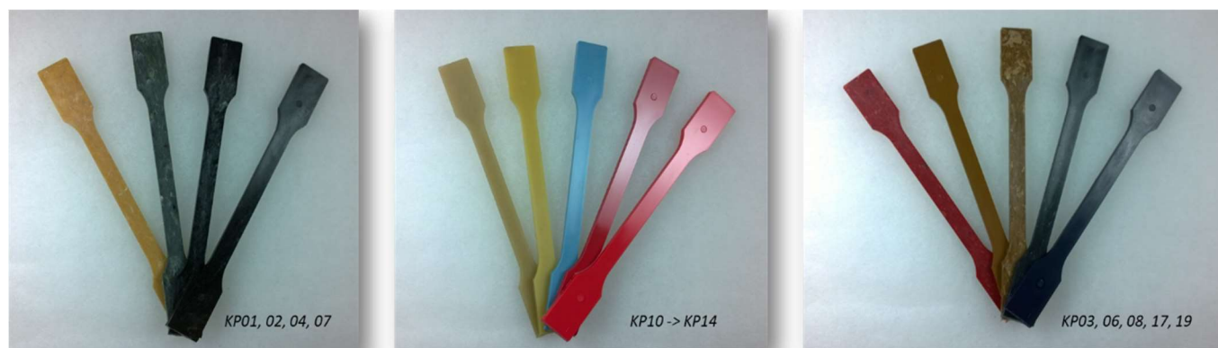
Figure 8 Plastic and composite rods made of various textile wastes (Heikkilä et al. , 2021)
