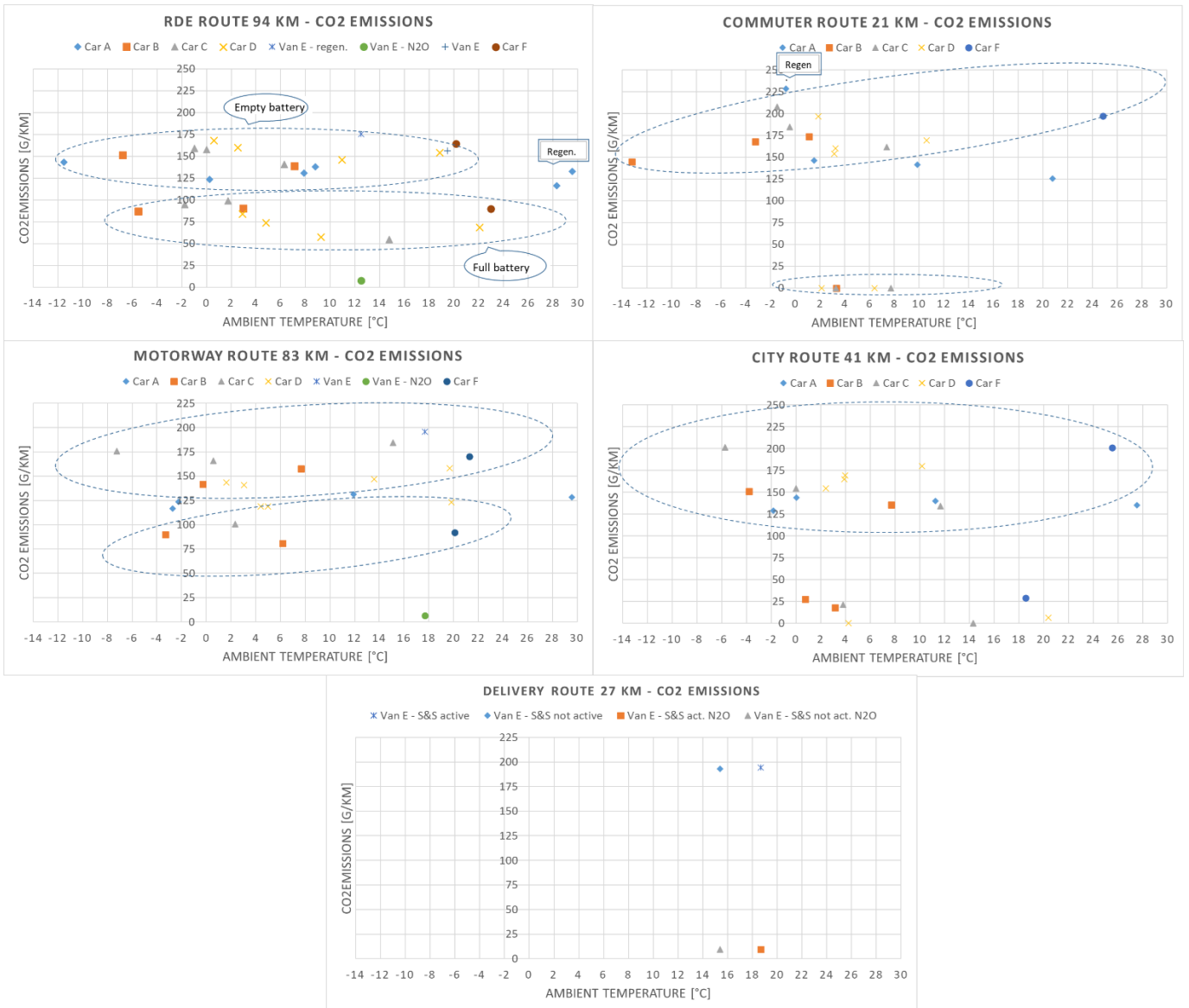
Figure 5: Trip average CO 2 emissions on test routes.
