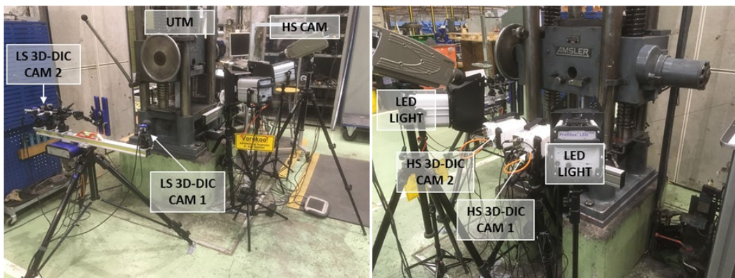
Figure 60: Test arrangements for the IWSLJ coupon static tests [107]. HS = high-speed camera, LS = low-speed camera. Figure courtesy of VTT.
