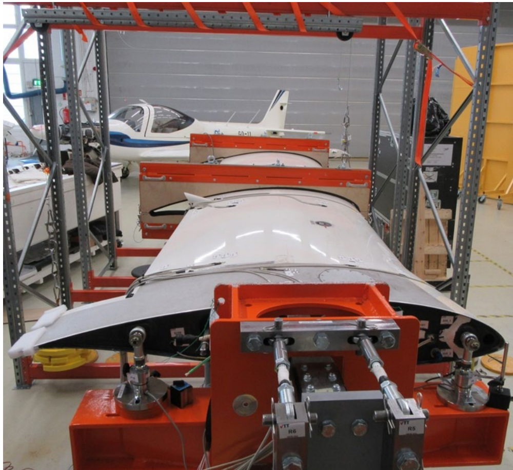
Figure 19: One of the load cases of the tested left wing. Figure courtesy of Patria Aviation.
