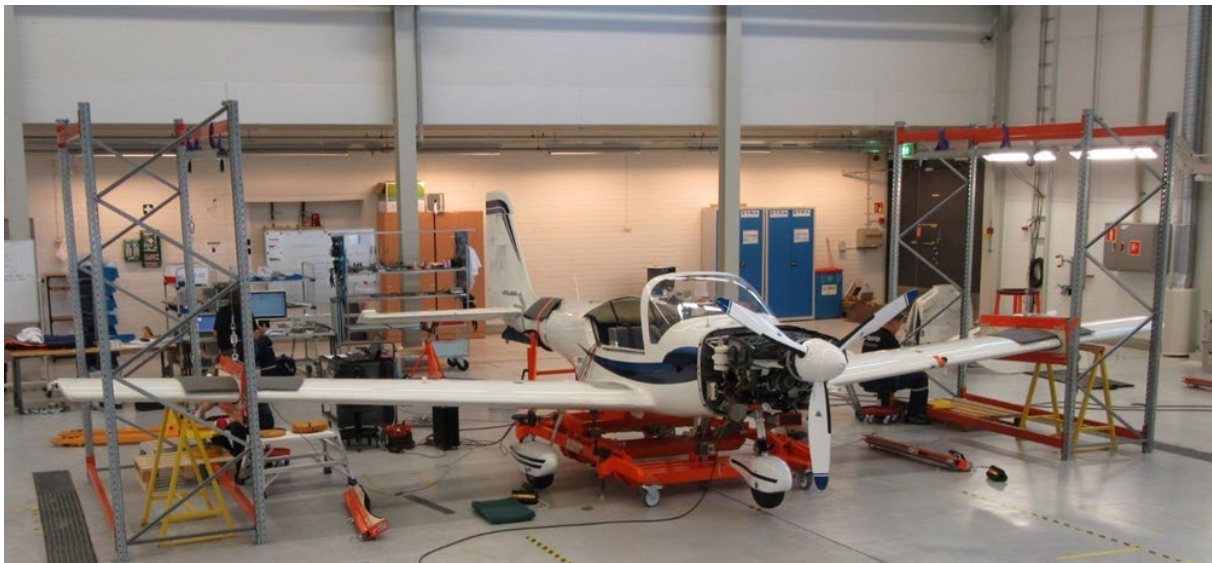
Figure 18: Calibration of the wing strain channels of the instrumented Grob G115E aircraft. Figure courtesy of Patria Aviation.
