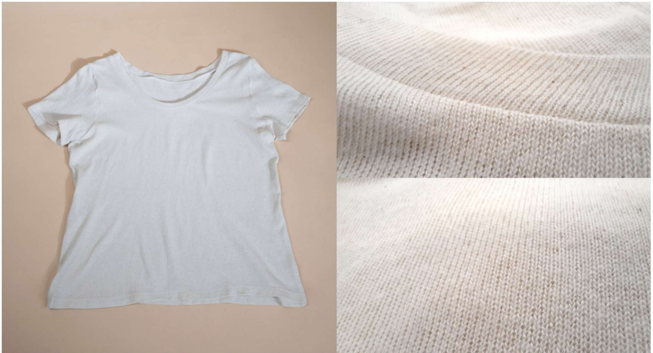
Figure 20 T-shirt yarn: 60% mechanically opened r-CO 40% r-PET, 20 Ne, (33 Nm, 30 tex), Pure Waste.
