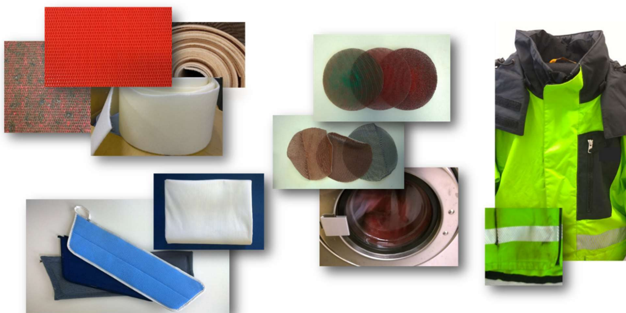
Figure 23 Examined sample materials. Majority content in the samples was either polyester (PET) or polyamides.
