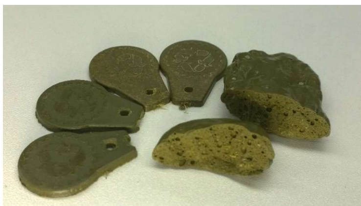
Figure 25 Demo samples from work clothes and damage caused by moisture intake (swelling/foaming).
