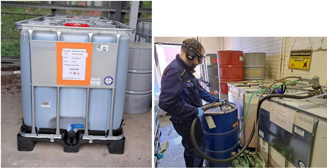
Figure 10 Photo of the fuel tank doped with the lube (left hand side) and preparing the lube mix to fuel (right hand side).
