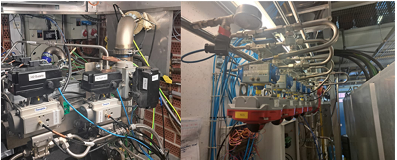
Figure 28: Test automation components for controlling the Nitrogen and Hydrogen feed into the engine.
