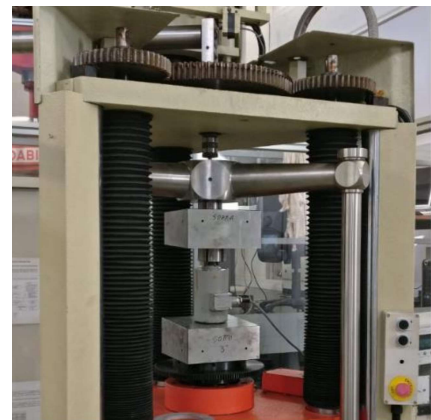
Figure 3 Investigation of the influence of spurious side forces and bending moments using tilted plates
