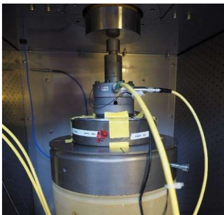
Figure 2 Investigation of a force transducer at different temperatures using a climate chamber
