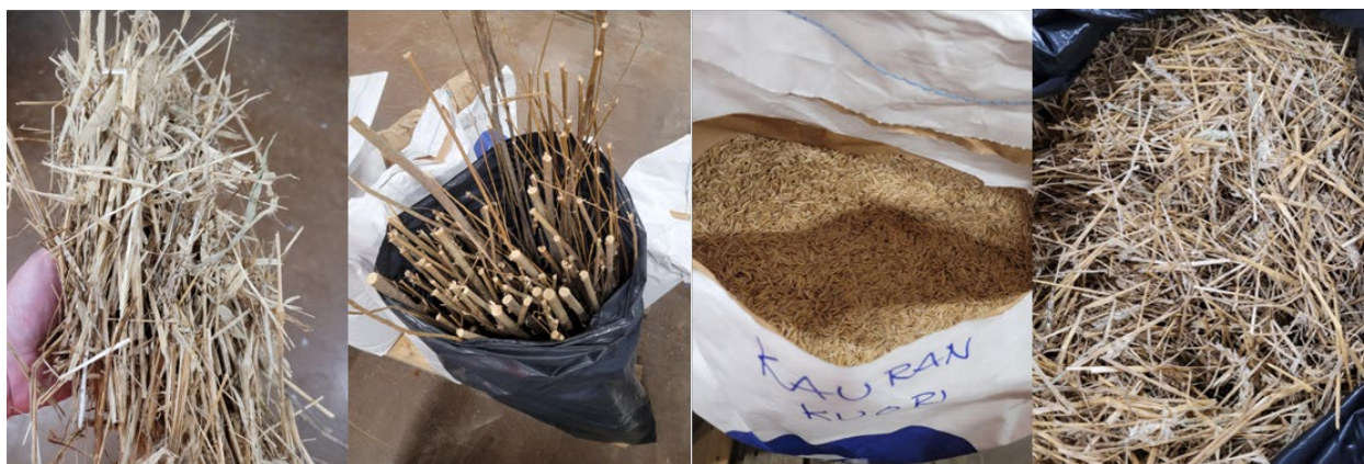
Figure 3. Used raw materials in the project from left to right: wheat straw, willow, oat husks and reed canary grass.
