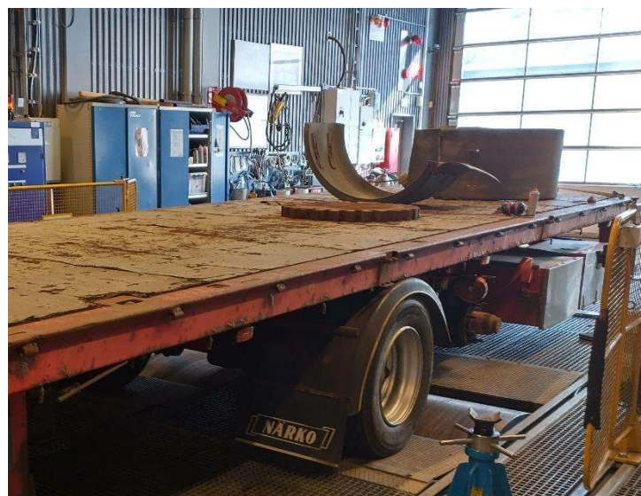
Figure 5. Trailer test rig used for tires with 19.5" rims.
