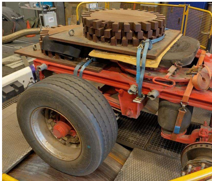
Figure 4. Dolly test rig used for tires with 22.5" rims.
