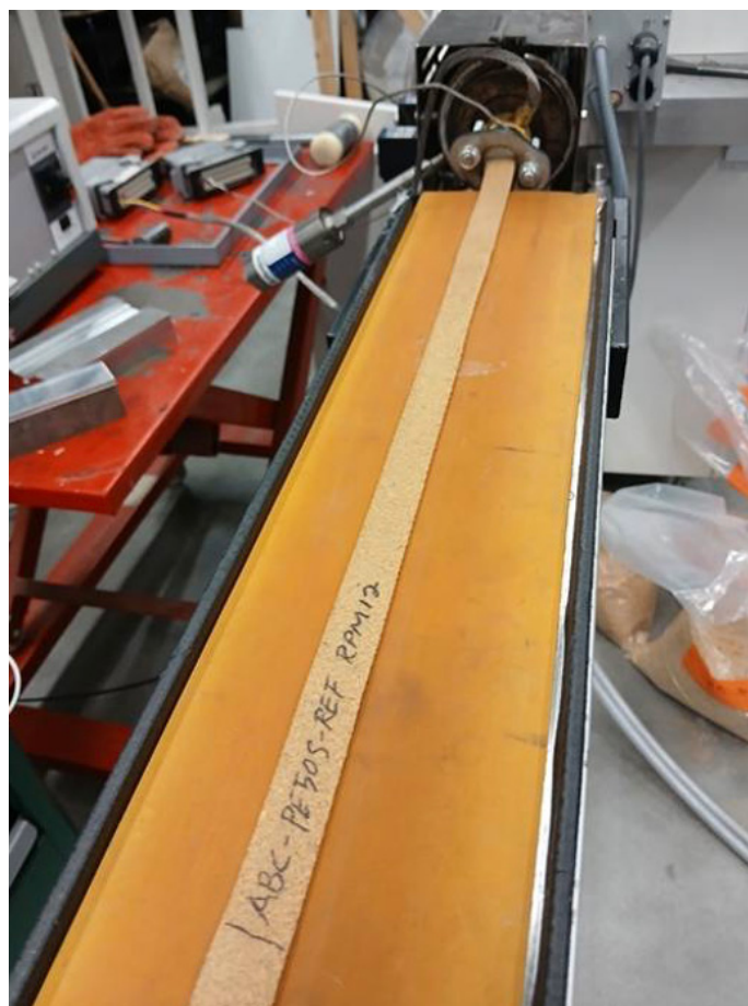
Figure 31. A single-screw laboratory extruder with a flat die producing PE with a 50 wt% sawdust composite profile. (Image Kusti Ruokamo)
