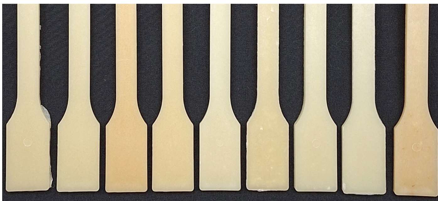
Figure 21. Injection-moulded samples containing additives for improved fibre dispersion and improved hydrophobic properties. All samples contain 20% of BSKP fibre in bio-LDPE.
