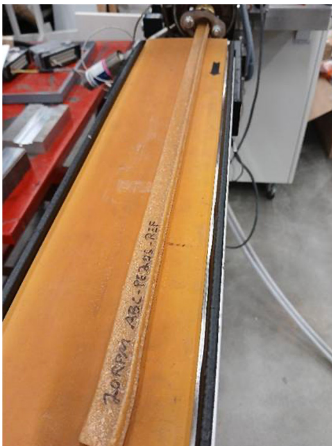
Figure 30. A single-screw laboratory extruder with a T-shape die producing a bio-LDPE with a 20 wt% sawdust biocomposite profile. (Image Kusti Ruokamo)
