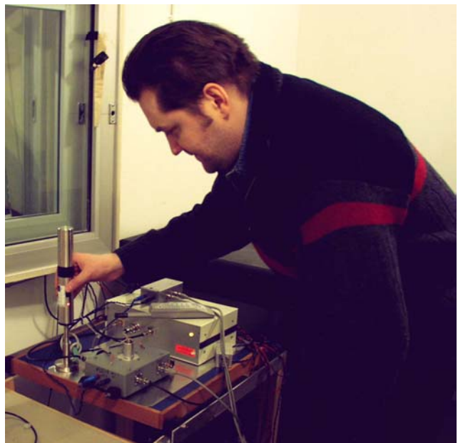
Kari Ojasalo performing pistonphone calibration in the new National Standards Laboratory of sound pressure.
