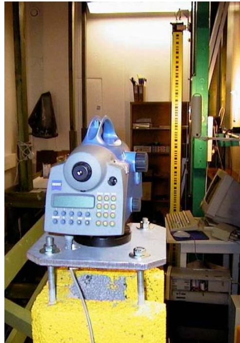
Automatic calibration of the Zeiss DiNi12 digital levelling system.
