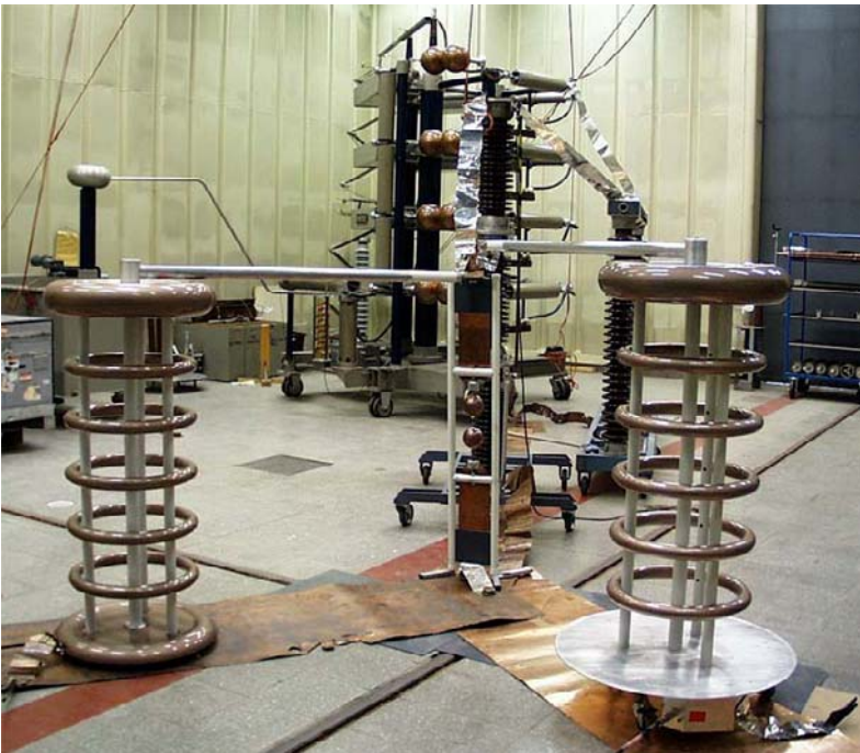
Measurement arrangement in 400 kV lightning impulse voltage comparison.
