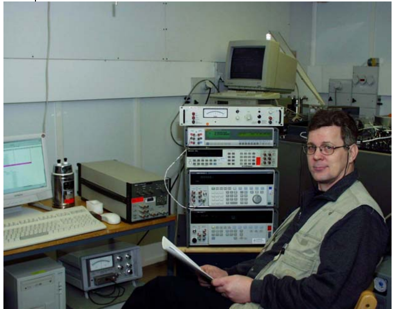
Risto Rajala performing a calibration using new instruments, Fluke 5720A calibrator and Fluke 8508A reference multimeter.
