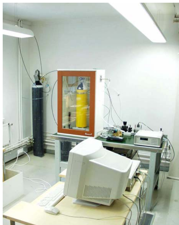
Overview of the MIKES calibration system for small gas flow meters.
