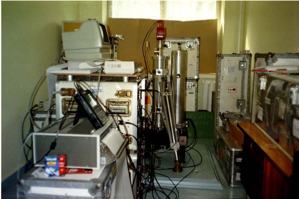
Absolute gravity measurement with the JLAg-5 in Panevėžys, Lithuania.
