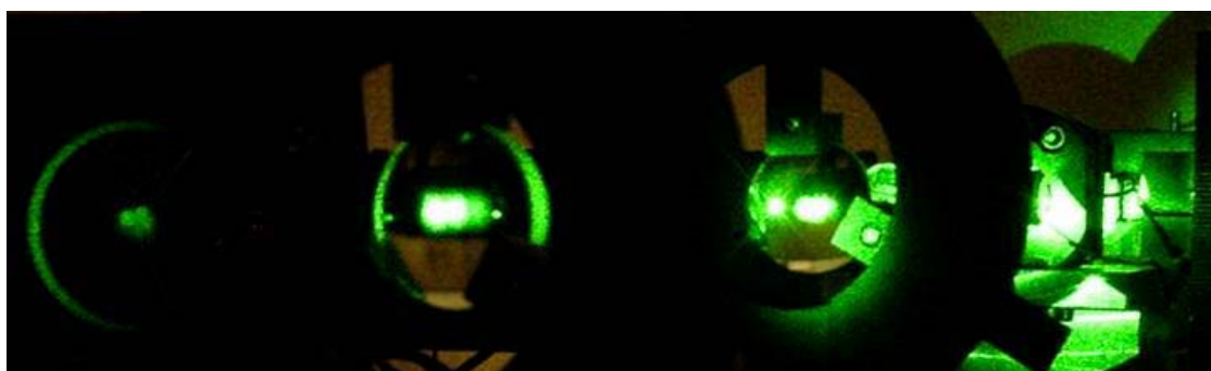
Frequency-doubled Nd:YAG laser emits green light at a wavelength of 532 nm.
