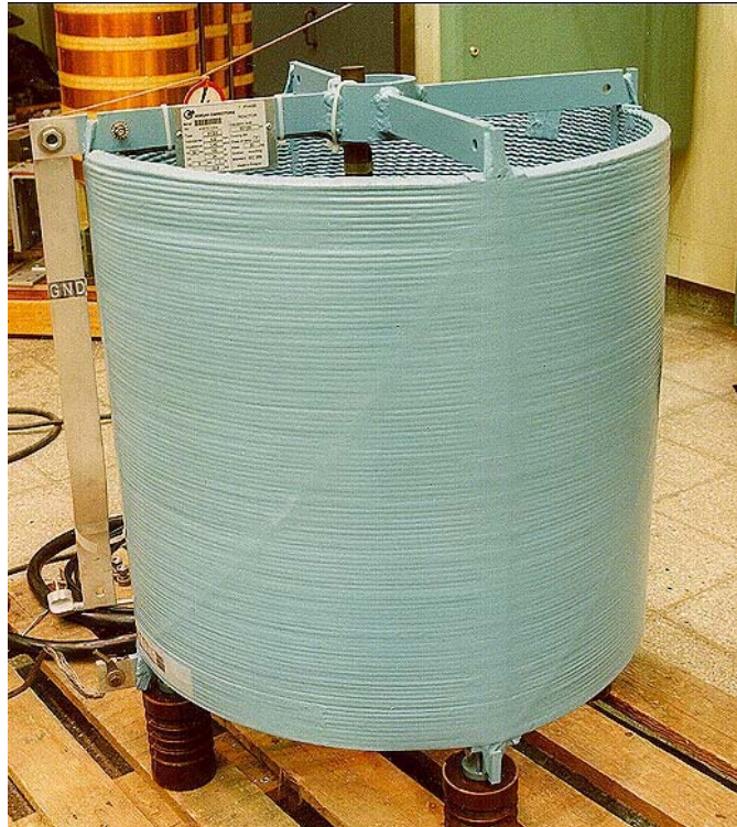
Reference coil for inductance comparison (4 mH, Q \approx 15 ). It is about 70 cm high and weighs about 50 kg.
