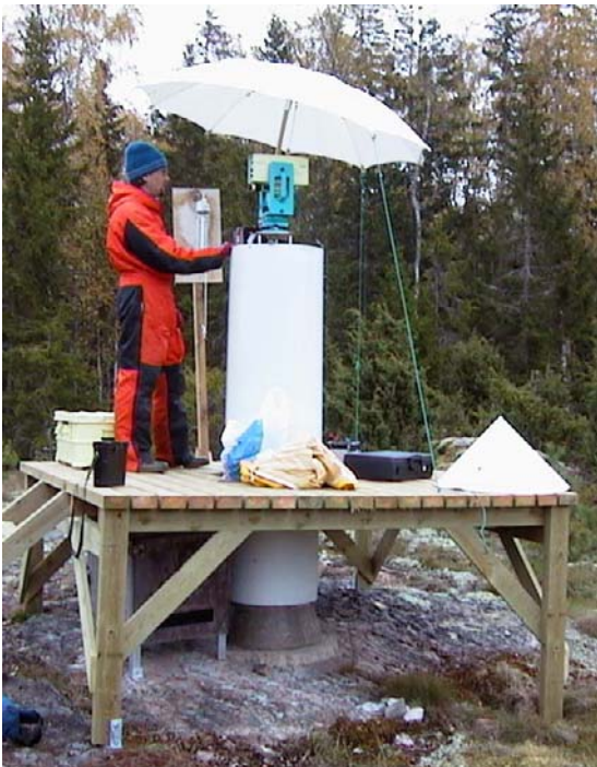
Controlling the scale of a local GPS network with high precision EDM.
