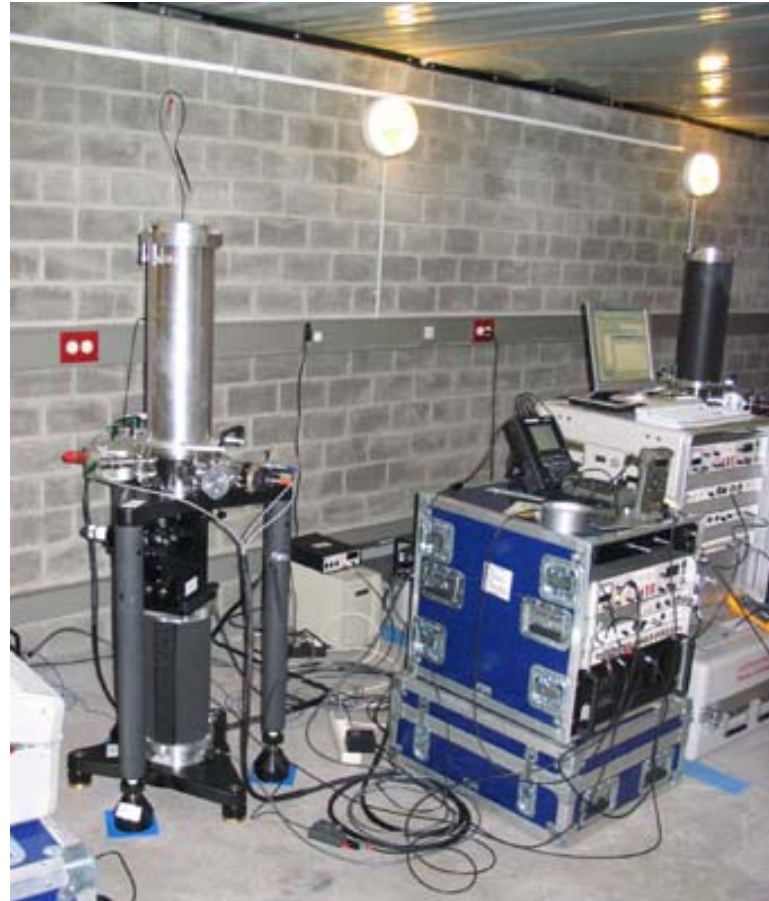
Figure M4. The FG5-221 of the FGI, here photographed at the International Comparison of Absolute Gravimeters in Luxembourg with another FG5 in the background. On the left (from top to bottom) the dropping chamber, the interferometer and the super spring. On the right the blue electronics rack.
