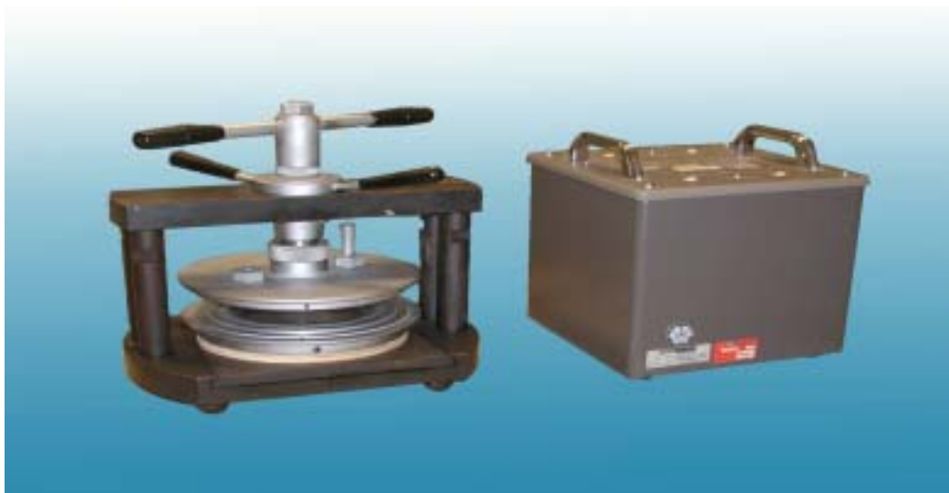
Figure E7. A variable guard ring capacitor (left) was used to calibrate the absolute losses of a 100 pF reference capacitor (right). Calibration was performed at power frequency (50 Hz), voltage was some hundreds of volts.
