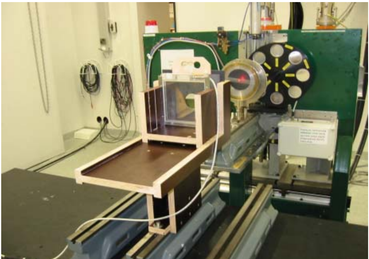
Figure I2. A test set-up for the calibration of DAP meters at the X-ray beam facility of STUK.
