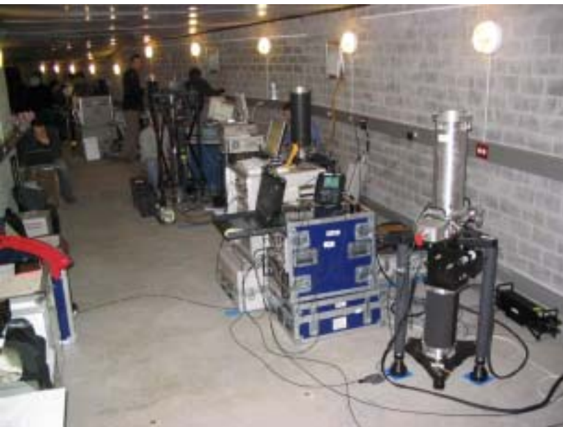
Figure. M8. A view from the International Comparison of Absolute Gravimeters in Luxembourg. Behind the FG5-221 of the FGI, the FG5-209 of METAS and the IMGC-2 of IMGC can be discerned. Twelve more gravimeters are mounted in the laboratory that was built in the gallery of former gypsum mine. Each gravimeter occupied three different sites during the comparison.
