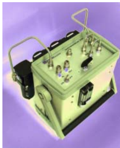
Figure T4. The humidity control unit of the calibrator constructed for Orion Pharma.
