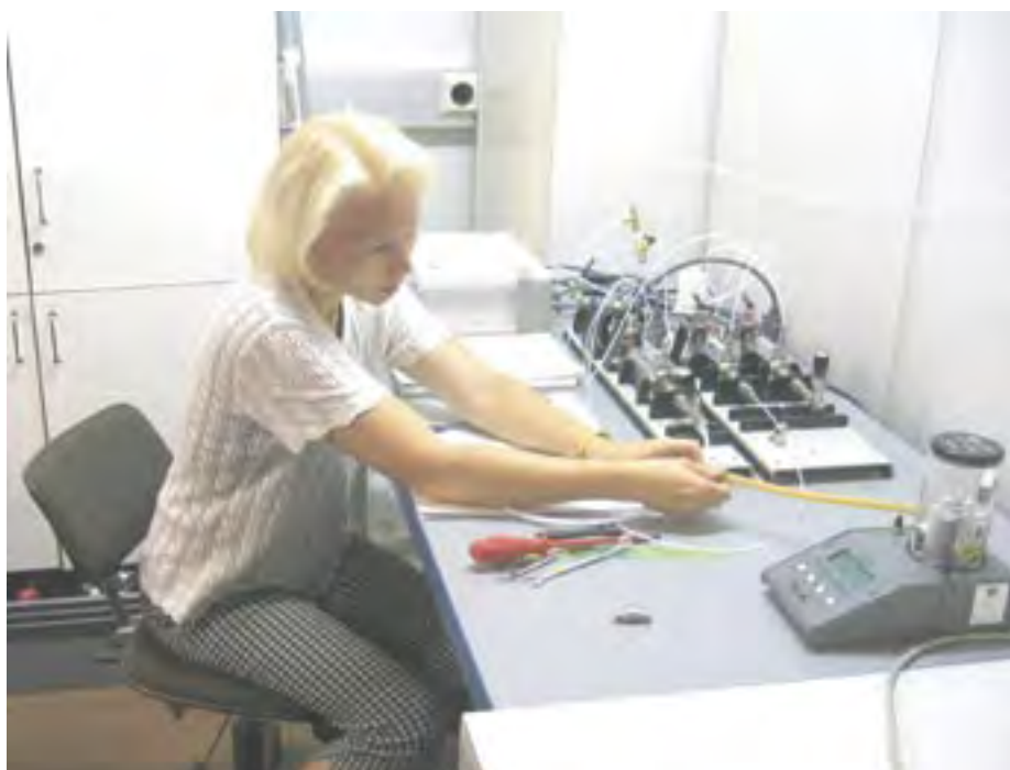
Figure C3. Kaisa Lusa is calibrating the flow meter with the DHI-laminar flow element. The flow measurement system is used for calibration of the flow measurement devices (e.g. mass flow controllers) and the gas dilution devices.
