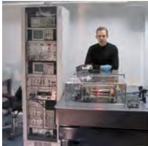
Figure L4. Mikko Merimaa presenting the ventilated rack enclosure for control electronics of the 633 nm HeNe lasers.
