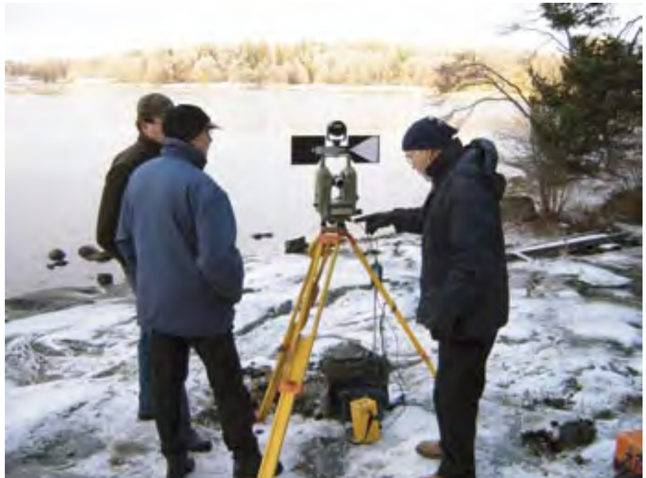
Figure L12. Preparing for water crossing with precise trigonometric levelling.
