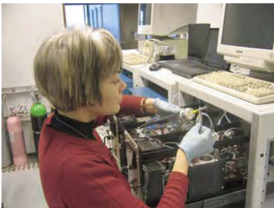
Figure C2. Sisko Laurila is operating the permeation method for calibration purpose of NO x , SO 2 , benzene, toluene, o- and m-xylenes.
