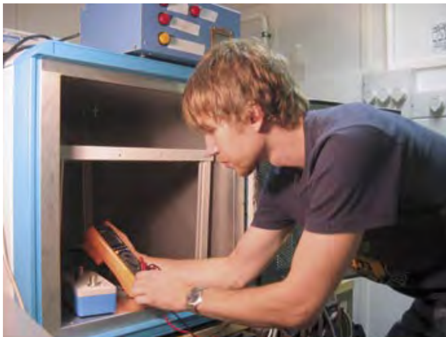
Figure E7. Pekka Sipilä preparing for measurements of 1 T \Omega resistance standard using the self-constructed temperature controlled enclosure.
