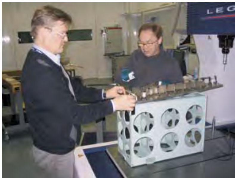
Figure L6. Adjustments for error mapping of new Mitutoyo LEGEX 9106 at 07PIT by experts of seller.
