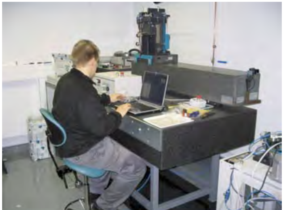
Figure L9. Antti Korhonen is working on a new device for squareness measurements for his thesis.
