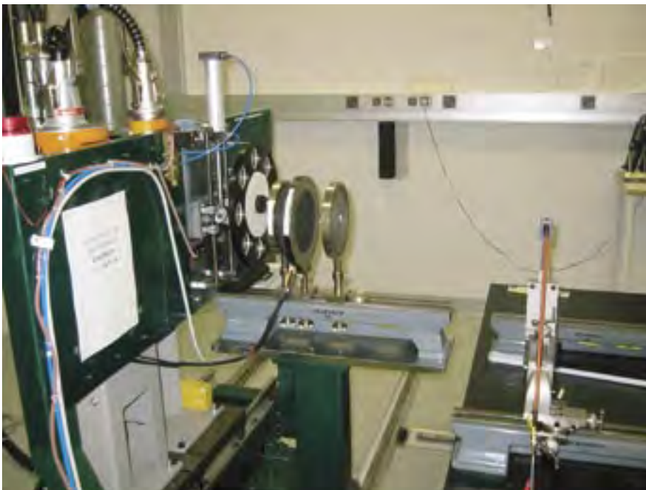
Figure 11. Measurement set-up for measurement of half value layers for x-ray radiation beams.
