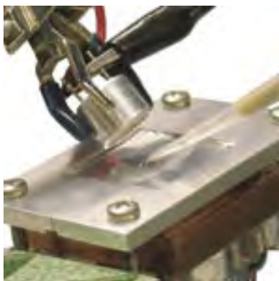
Figure T6. Studying the effect of ultrasound and electric field on freezing of a supercooled water droplet.
