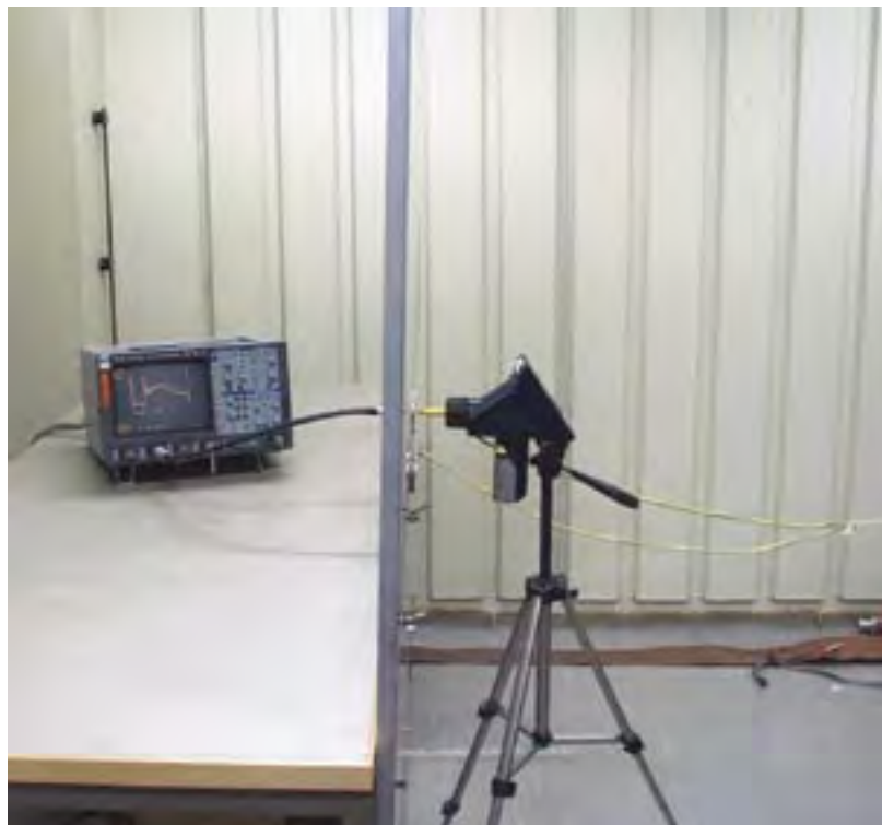
Figure E9. ESD-tester (on the right) is calibrated using a target mounted on a conducting plane. The signal is measured by a wide-band oscilloscope. MIKES-TKK participated in an informal comparison in October 2005.
