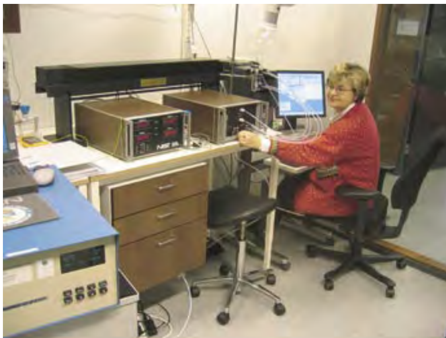
Figure C1. The Standard Reference Photometer (SRP no 37) by NIST for ozone calibration. The traceability of the ozone concentration is to BIPM by direct comparison of the two SRPs by NIST. Dr Pirjo Kuronen is preparing the calibration.
