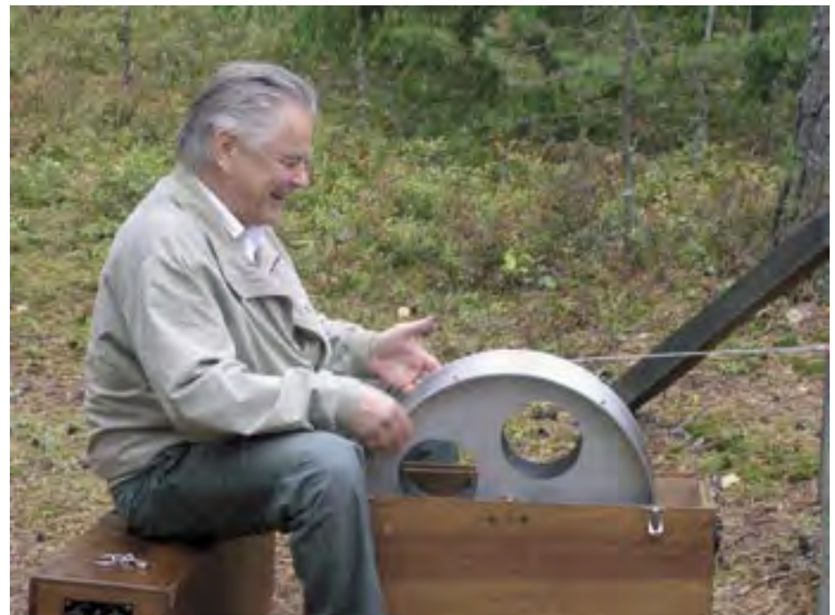
Figure L12. The FGI has made documentary films to preserve the heritage of old measurement skills and methods. Here Professor (emeritus) Jussi Kääriäinen demonstrates the use of invar wire at the Nummela Standard Baseline.
