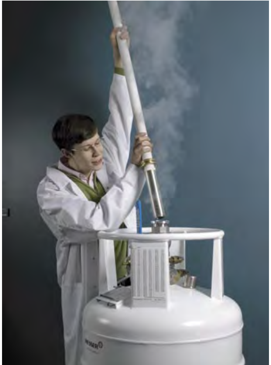
Figure E3. Ville Maisi experimenting with the new cryoprobe for AC voltage and power quantum standards. The new probe exhibits a minimal liquid helium boil-off rate of about 1 litre/day.
