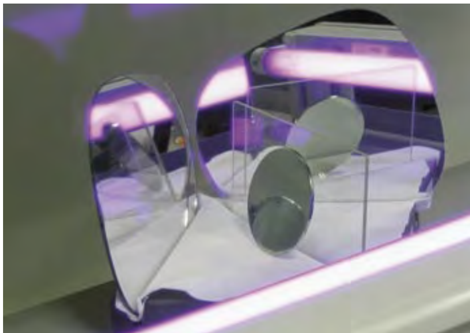
Figure T1. TiO 2 coated stainless steel plate is being irradiated with ultraviolet light. The ultraviolet light is supposed to dissolve biological compounds due to catalysis on the surface with photo-electrochemical reaction.
