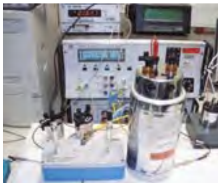
Figure E6. Measurement of the 1 G \Omega travelling standard from the MIKES reference 100 M \Omega standard in EUROMET.EM-K2 comparison by two methods: DCC resistance bridge (left) and modified Wheatstone bridge based on two calibrators (right).
