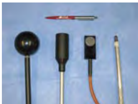
Figure 12. Set of ionisation chambers. Second from right, 23344-type plane parallel chamber used as a reference standard for x-rays.
