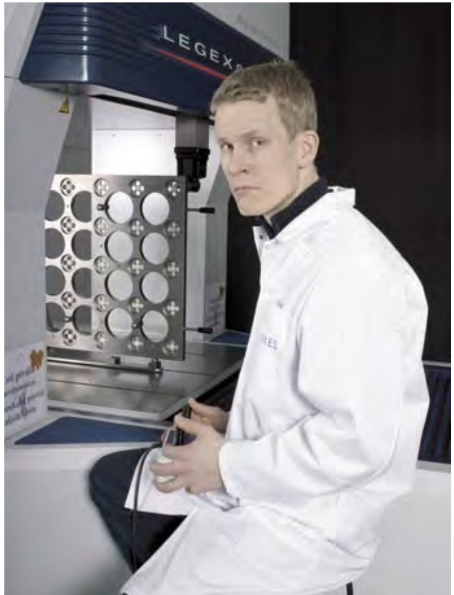
Figure L10. Ilkka Palosuo is performing error separation measurement with a ball plate and CMM.
