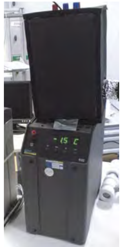
Figure T7. Portable humidity calibrator developed at MIKES.
