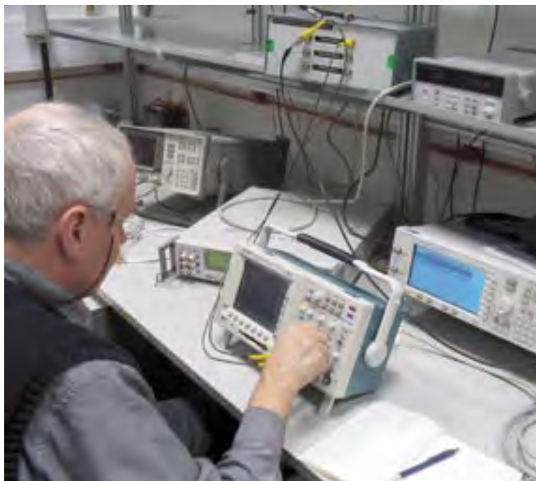
Figure E7. Kalevi Kalliomäki investigating the transfer standard of comparison EUROMET.TF.TI-K1. The transfer standard (middle up) consists of three microwave cables of different lengths fitted in a box and equipped with BNC connectors.
