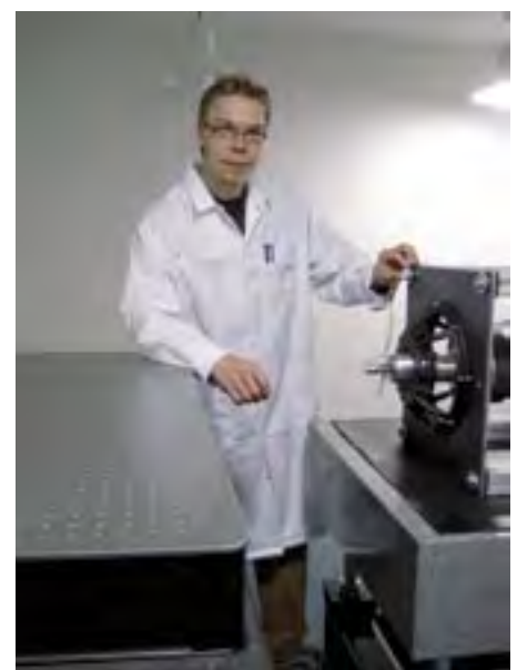
Figure E4. Jussi Hämäläinen testing the accelerometer comparison setup, which is based on a homemade shaker.
