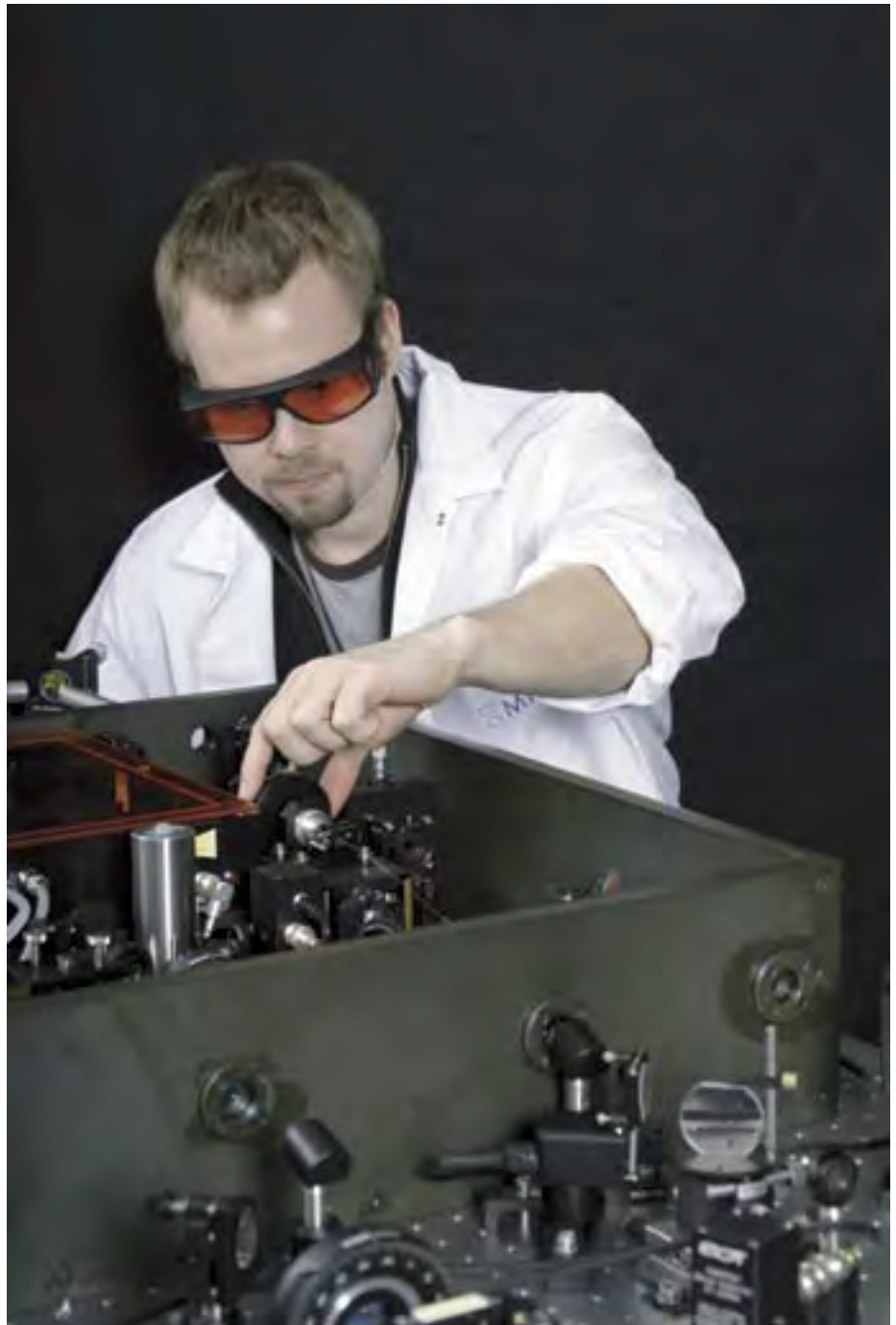
Figure L1. Ville Ahtee adjusts the frequency comb generator. (Photo: M. Merimaa)
