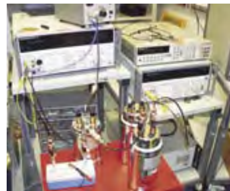
Figure E6. Measurement of the 1 G \Omega travelling standard from the MIKES reference 100 M \Omega standard in EUROMET.EM-K2 comparison by two methods: DCC resistance bridge (left) and modified Wheatstone bridge based on two calibrators (right).
