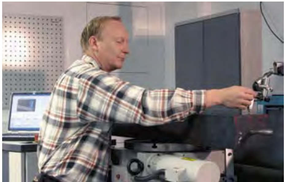
Figure L8. Asko Rantanen is adjusting squareness measuring instrument.
