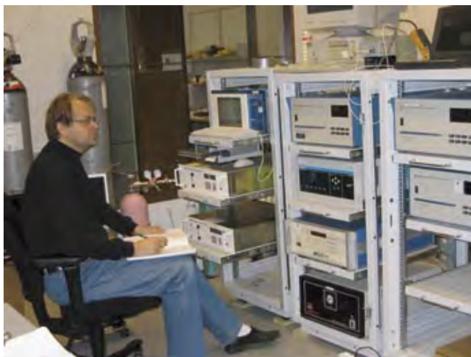
Figure C2. Antti Wemberg is obtaining calibration of continuous air quality analyzers of oxides of nitrogen, sulphur dioxide and carbon monoxides.
