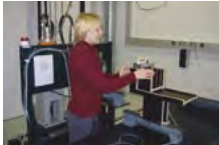
Figure 11. Calibration of a kerma area product meter with x-rays.
