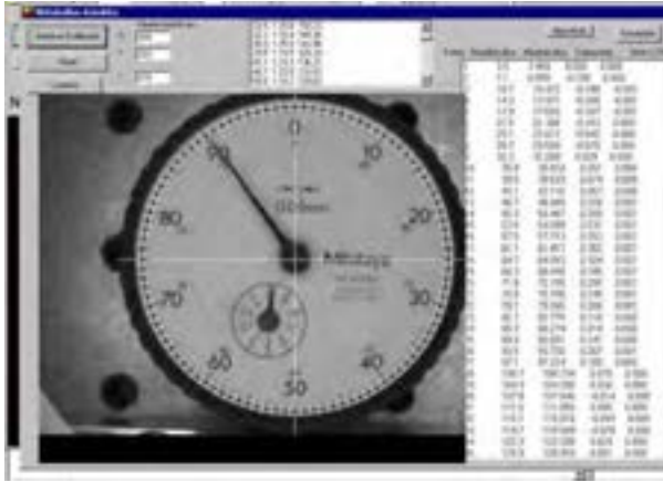
Figure 5. Measurement of the scale marks on the dial.
