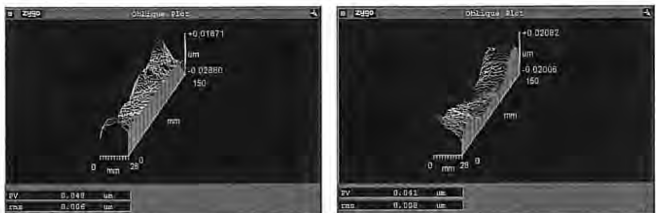
Figure 6. Flatness deviations of the mirror surfaces (left x-axis mirror surface, right y-axis mirror surface).
