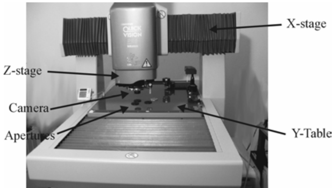
Figure 9. The optical CMM at MIKES.
