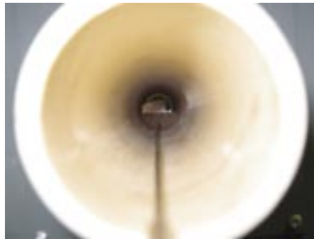
Figure T4. A silicon wafer ready for an emissivity test in a high-temperature furnace.
