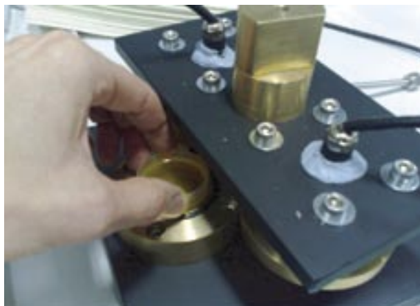
Figure T8. A honey sample located in the measurement chamber of the apparatus developed at MIKES.
