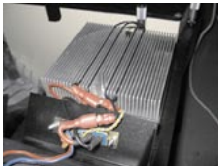
Figure P1. Modification of the current leads of the Peltier element. The positive current lead forms two loops that are placed in such an orientation that the magnetic field produced compensates for the magnetic field produced by the Peltier element.
