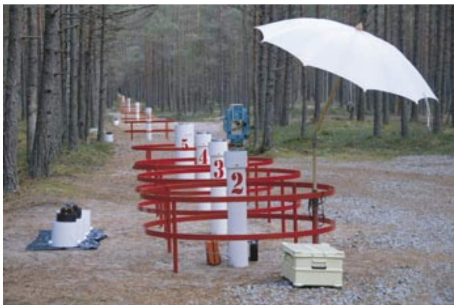
Figure L10. Vääna calibration baseline in Estonia.
