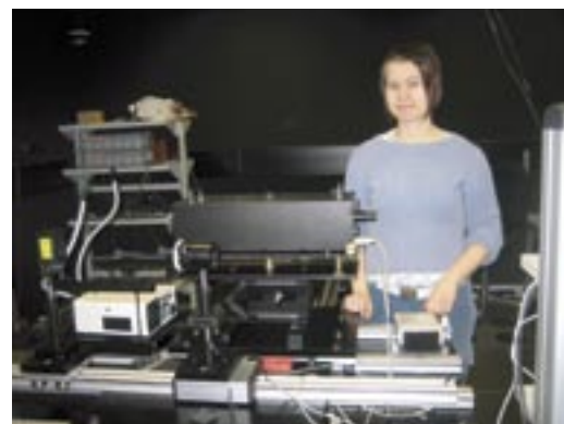
Figure T3. Maija Ojanen comparing a filter radiometer to a linear pyrometer.
