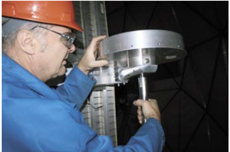
Figure L11. Installing a GPS antenna for tie measurements in the 14 m high VLBI telescope at Metsähovi.
