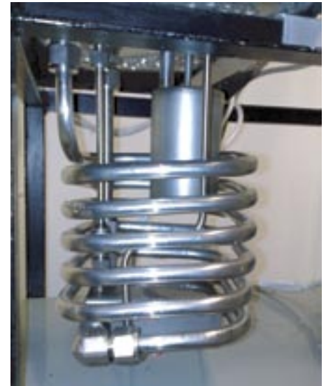
Figure T5. The High-Range Saturator designed and manufactured for FSB-LPM by MIKES.
