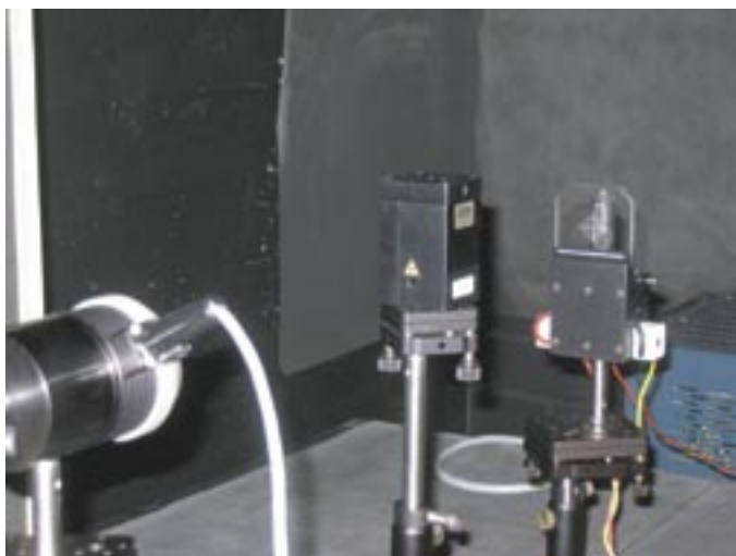
Figure P7. Aligning the detector and the lamp to the same optical axis using a two-output laser source.
