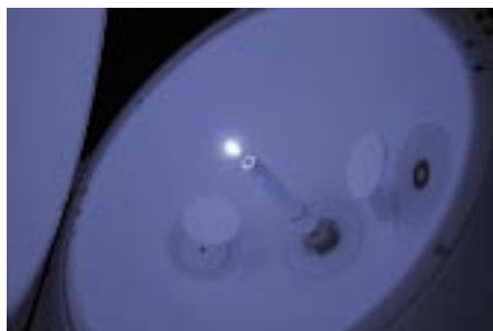
Figure P4. A photograph of a LED comparison measurement showing the new improved LED holder in operation. The screening due to the new holder is barely visible. Only the two baffles form shades inside the sphere, preventing the detector and auxiliary port from seeing the light source directly.
