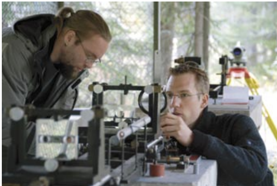
Figure L3. Pasi Häkli and Martin Rub are installing the Väisälä comparator for interference measurements at the Nummela Standard Baseline.
