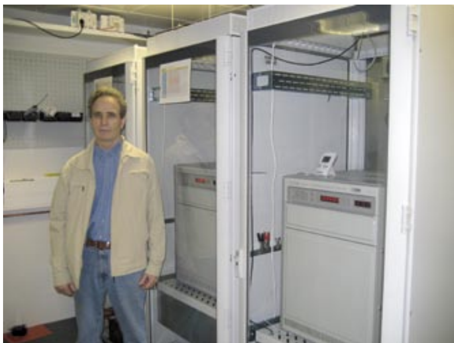
Figure E7. Dr. Nikolai Demidov from IEM KVARZ visited MIKES and made the final adjustments of the new active hydrogen maser CH1-75A in January 2008.
