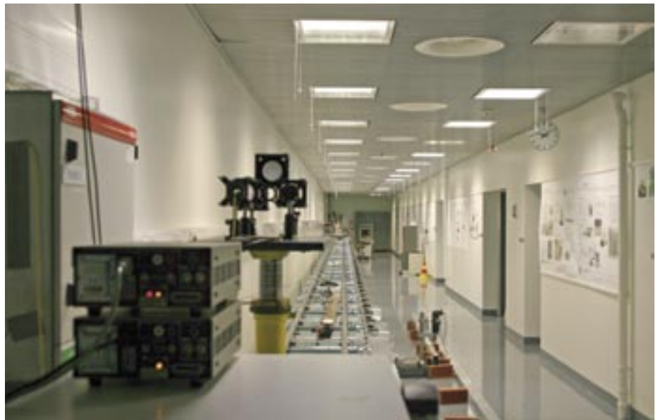
Figure L7. Test setup for spectroscopic air temperature measurement on MIKES 30 m interferometric bench.
