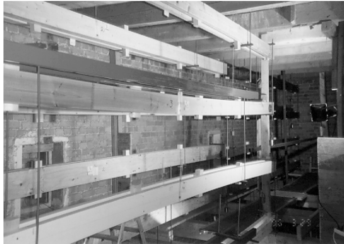
Figure 1. Photograph of test set-up and loading arrangements in sheltered environment.
