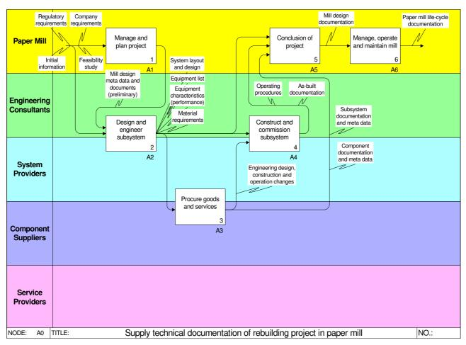
Figure 5. Main process diagram in the rebuilding of paper mill.
