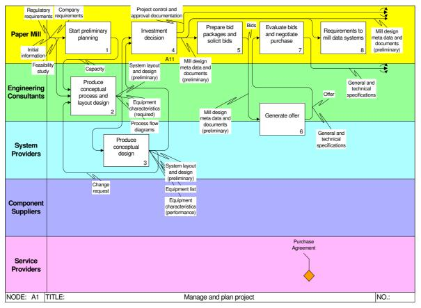
Figure 6. Manage and plan the project. Bids and offers include technical data.
