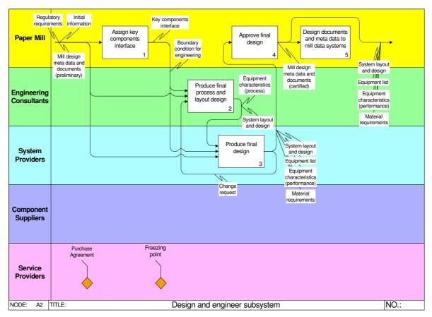
Figure 8. Design and engineer changes.
