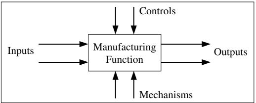
Figure 1. IDEFØ Function Box and Interface Arrows.
