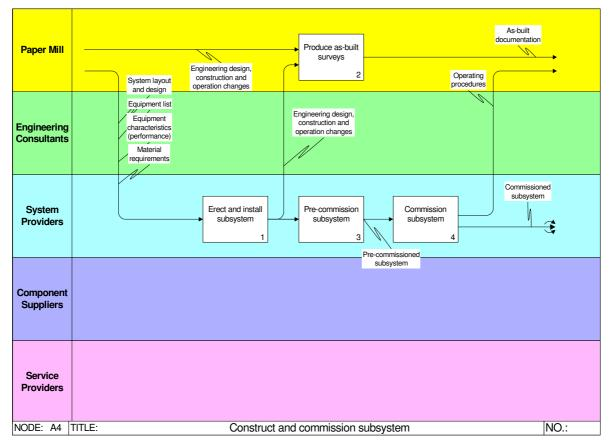
Figure 10. Construct and commission changes in the paper mill.
