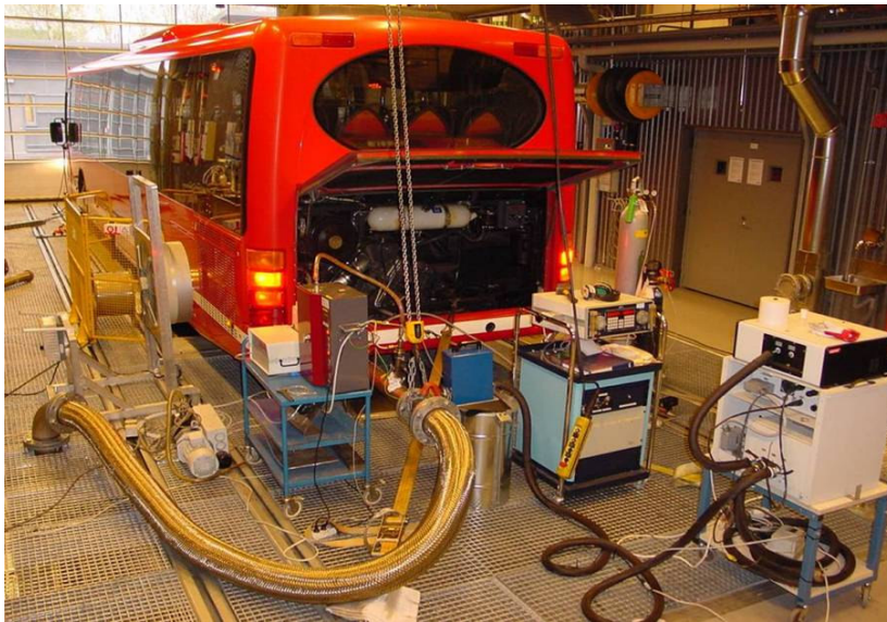
Figure 12. Emission testing of a bus on the chassis dynamometer.
