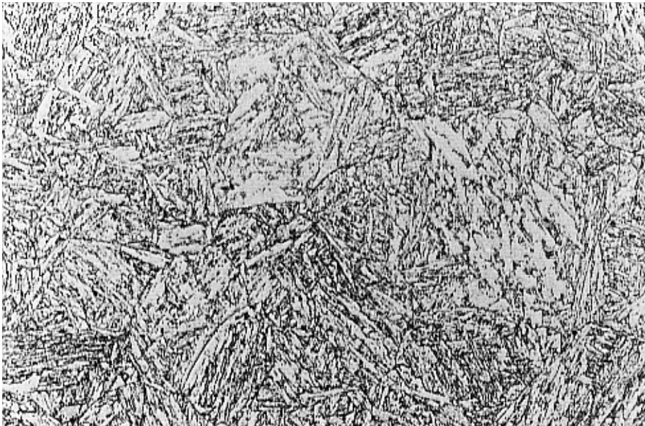
Fig. 38. Steel X 20 CrMoV 12 1: 780°C / 10 h, P_{LM} (C = 14) = 15\ 800 , stage C. Magnification 500x.
