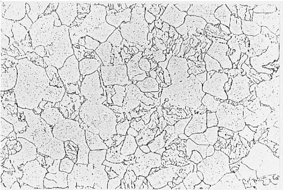
Fig. 30. Steel 10 CrMo 9 10: 720°C / 100 h, P_{LM} (C = 14) = 15\ 900 , stage D. Magnification 500x.
