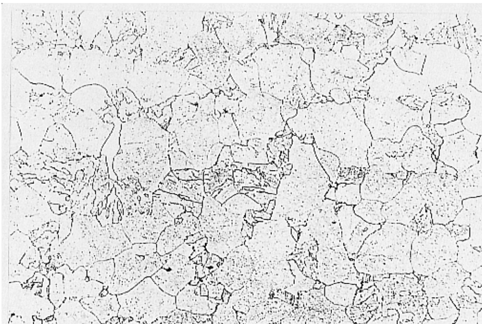
Fig. 28. Steel 10 CrMo 9 10: 720°C / 10 h, P_{LM} (C = 14) = 14\ 900 , stage C. Magnification 500x.
