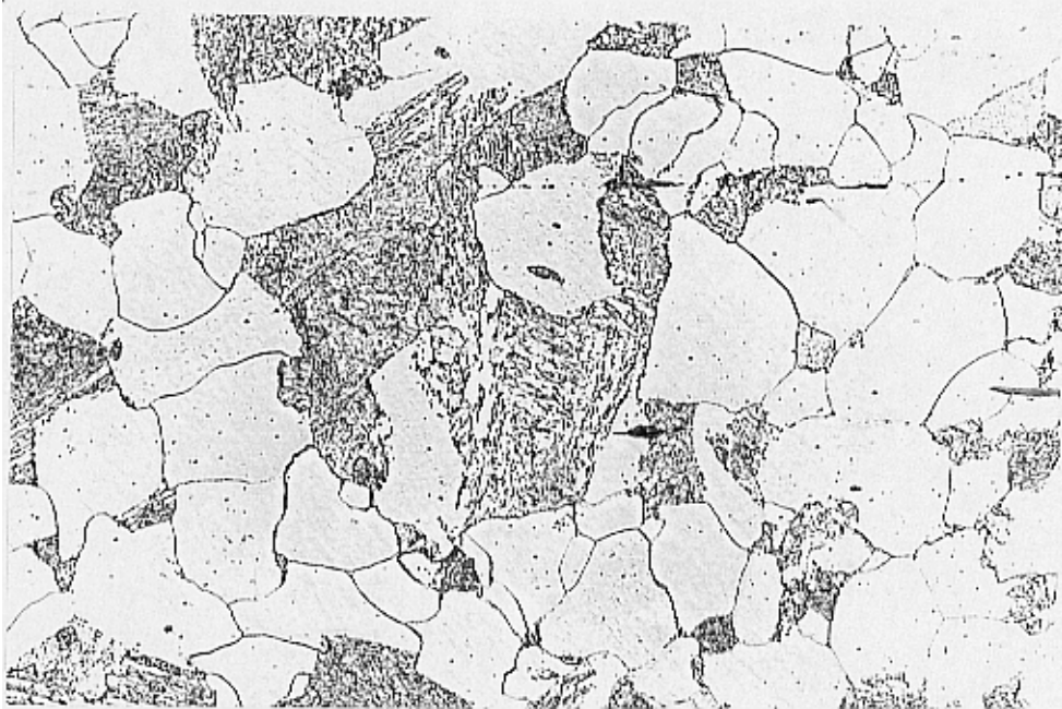
Fig. 19. Steel 13 CrMo 4 4: 720°C / 10 h, P_{LM} (C = 12) = 12\ 900 , P_{LM} (C = 14) = 14\ 900 , stage C. Magnification 500x.
