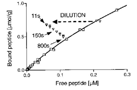
Figure 6. Part of an adsorption isotherm for  ${}^3H$  labeled CBHI CBD on BMCC ( $\Box$ ). In a dilution experiment several samples which had reached equilibrium were diluted and then filtered at different time points. In this way the disruption of equilibrium and the subsequent establishment of a new equilibrium could be followed ( $\nabla$ ). This result shows that the binding is reversible and that the "ascending" isotherm is the same as the "descending" isotherm (Norde and Haynes, 1995).
