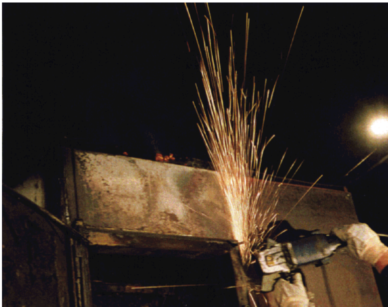
Figure 5. Experiment 3. A) fire cabinet, time after ignition 29.5 min, b) fire cabinet with ceiling ventilation openings blocked with soot, time after ignition 46.5 min, c) 3 days after the experiment, soot in the upper part of the cabinet was ignited by sparks when cutting open the welding seams between the rack and the cabinet frame.
