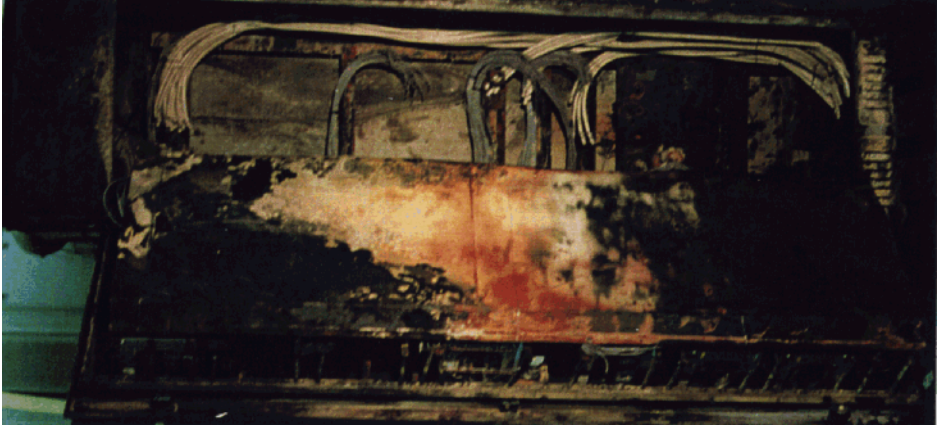
Figure 3. The fire cabinet before experiment 2. A) relays and circuit boards in the hinged rack, b) wiring on the left side wall leading to the relays in the hinged rack, c) wiring on the rear and vertical cable bundle on the left side wall.
