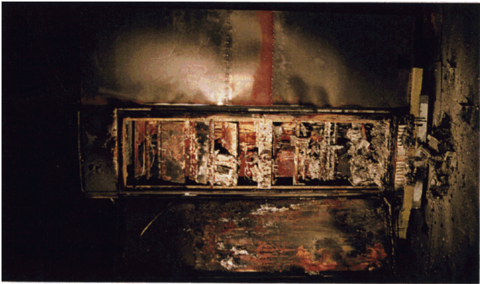
Figure 2. The fire cabinet after experiment 1. A) relays and circuit boards in the hinged rack, adjoining cabinet on the right, b) wiring on the left side wall, c) wiring on the rear, d) vertical cable bundle on the left side wall.
