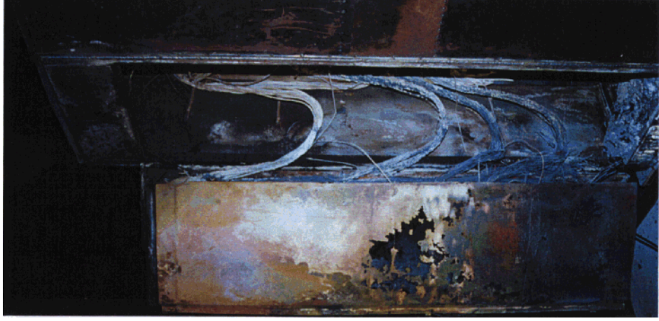
Figure 4. The fire cabinet after experiment 2. A) relays and circuit boards in the hinged rack, b) wiring on the left side wall leading to the relays in the hinged rack, c) wiring on the rear and vertical cable bundle on the left side wall.
