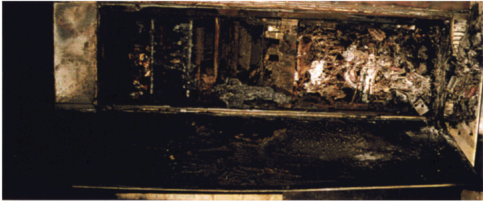
Figure 6. The fire cabinet after experiment 3. a) relays and circuit boards in the hinged rack, b) wiring at the rear and vertical cable bundle on the left side of the wall, c) the slab composed of melted plastics on the bottom of the fire cabinet has been broken while emptying the cabinet. Note the soot depositions in the upper part of the cabinet in a) and b).
