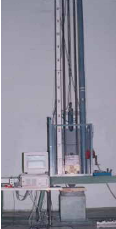
Figure 2. Instrumented falling weight impact tester.
