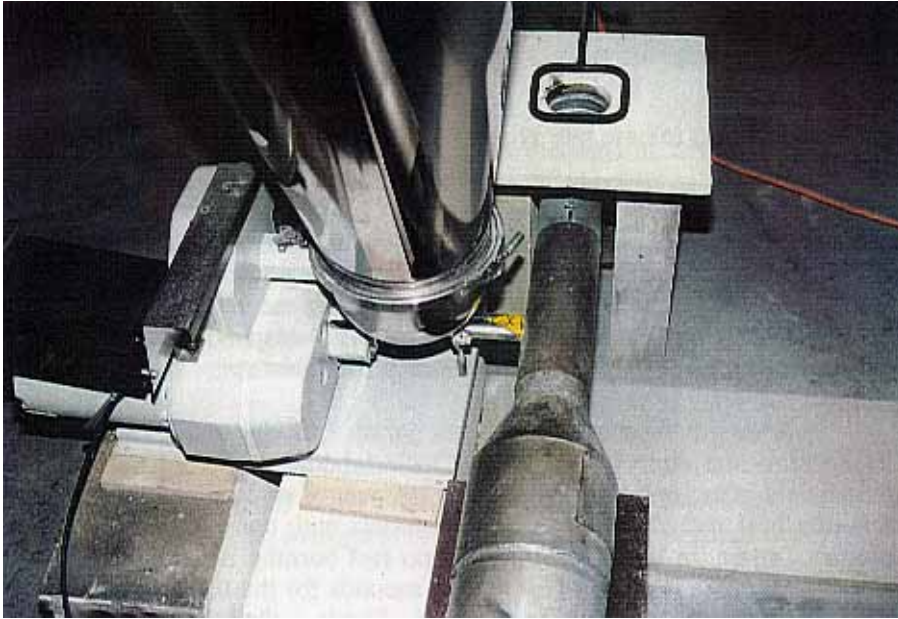
Figure 5. The powder feeder (left) is connected to the air stream line. The air blower is seen at the lower edge of the picture, and the gas burner on the Promatec plate centred around the air inlet hole at the upper edge.
