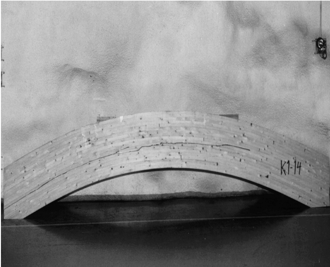
Failure behaviour of specimen LT-C2-S2-7.
