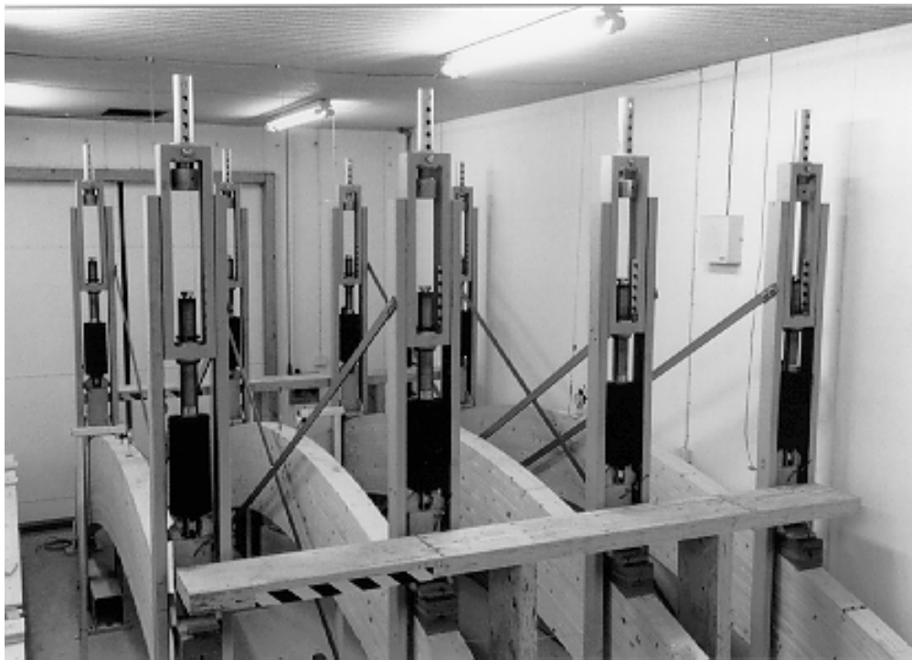
Figure 5. Photograph of specimens and loading springs for long term testing.
