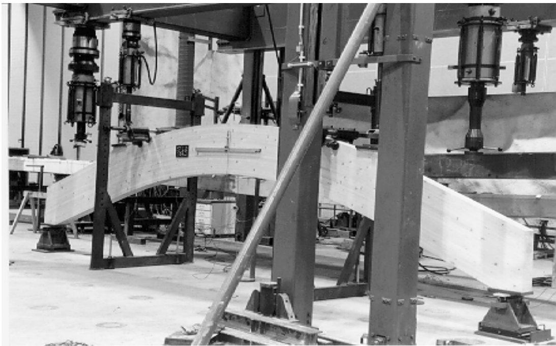
Figure 9. Photograph of test set up for short term tests: series ST-C2-S5b .
