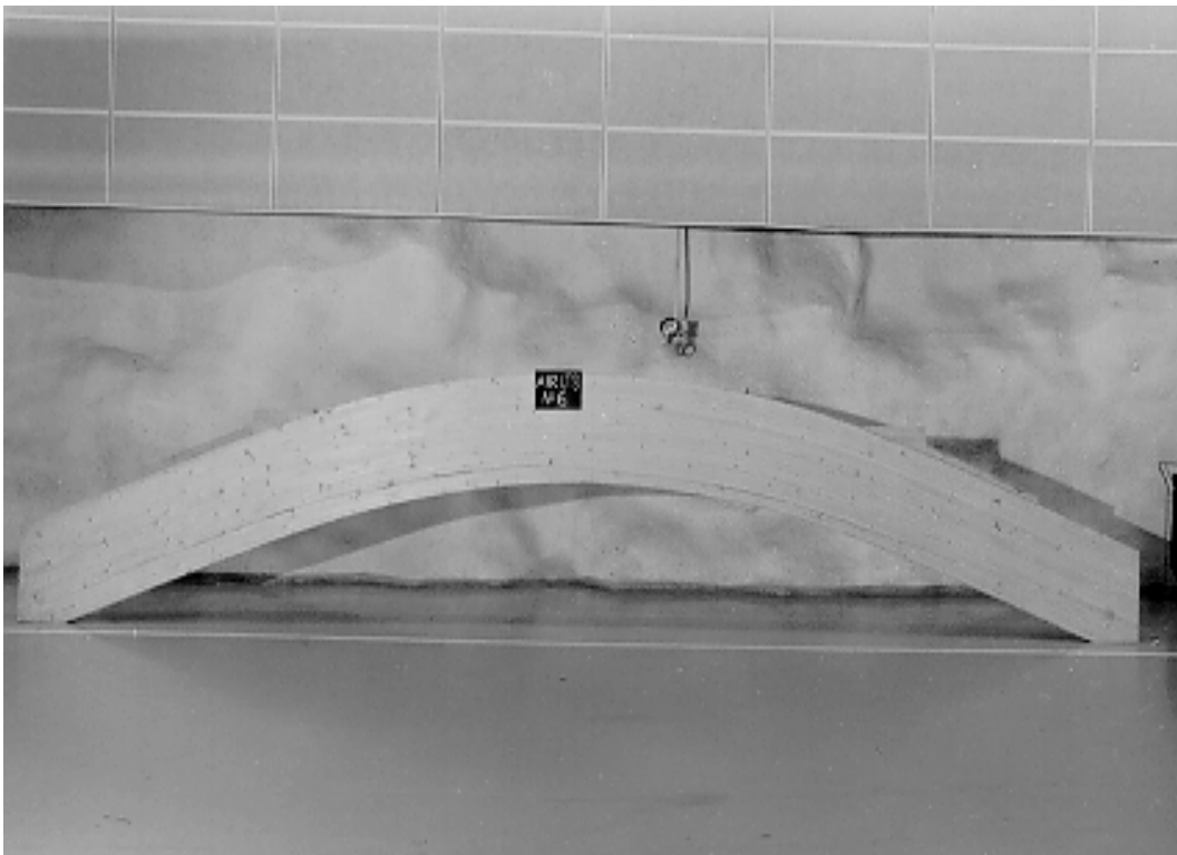
Failure behaviour of Specimen LT-C2-S4-6 (AIR LT3 No.6).
