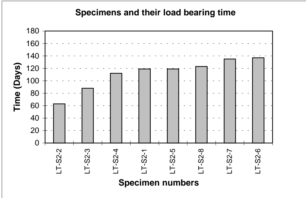
Figure 26. Variation of load-duration for specimens in series LT-C2-S2.
