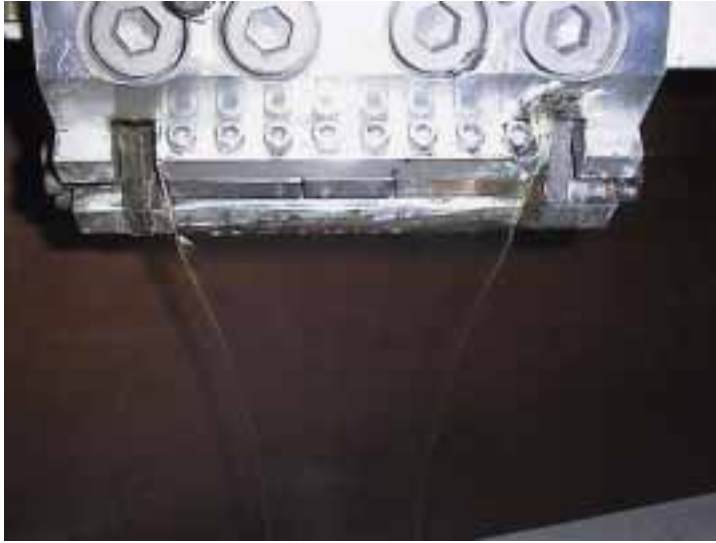
Figure 47. Solid film in flat die extrusion.
