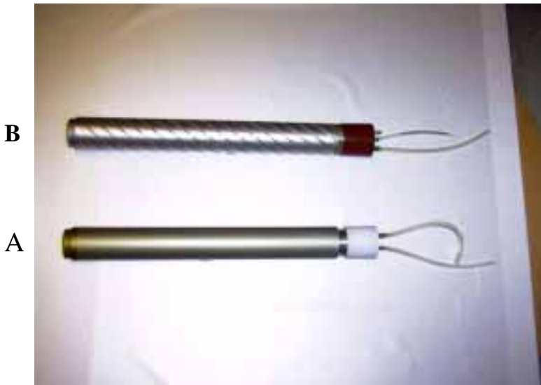
Figure 23. Water cooled mandrels for A) solid and B) foamed extrudate tube chilling.
