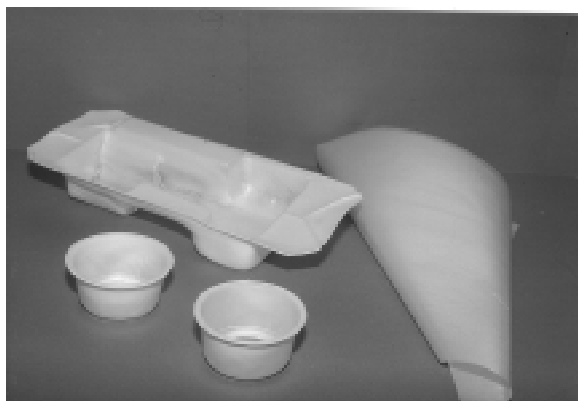
Figure 49. Thermoformed products and a sample of BOPP foam film. BimoPP
