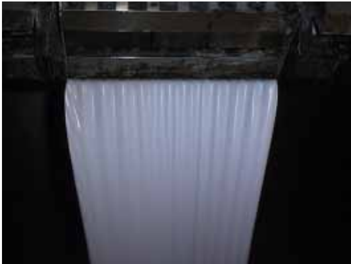
Figure 48. Foam film in flat die extrusion.
