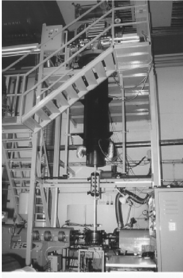
Figure 24. BOPP foam film line.
