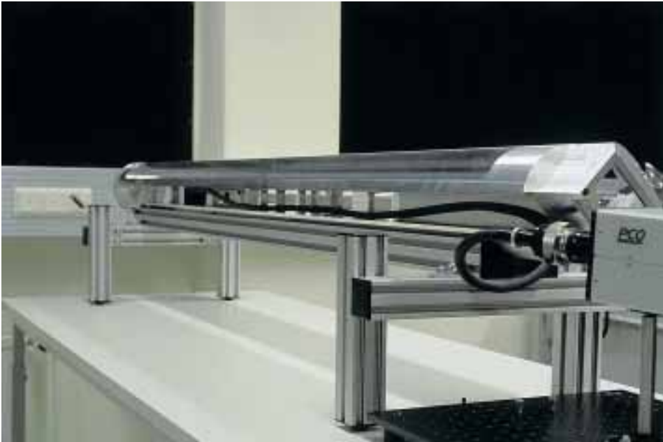
Fig. 4.6. The optical bench with CCD camera and optical fibre bundle.
