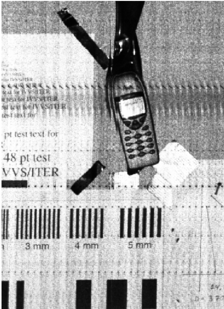
Fig.4.8. A test image (distance 2.5 m) obtained by rotating the view probe in steps.
