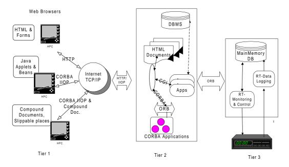
Figure 1. The 3-tier client/server architecture of the Open Object Web in embedded systems.
