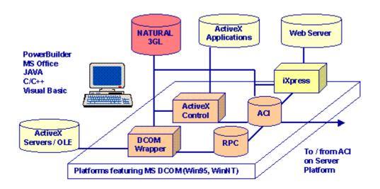
Figure 9. EntireX's components on typical client platforms.
