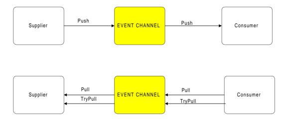
Figure 6. Event-based communication with push and pull models.
