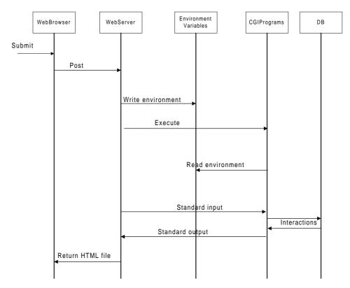
Figure 5. An end-to-end client/server scenario with CGI.
