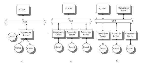
Figure 8. Alternatives for implementing object wrappers.
