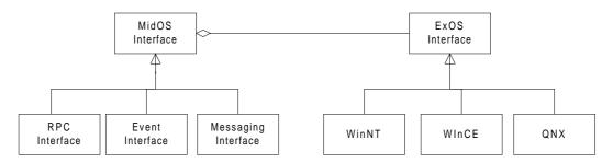
Figure 12. Isolating the impact of the execution environment.
