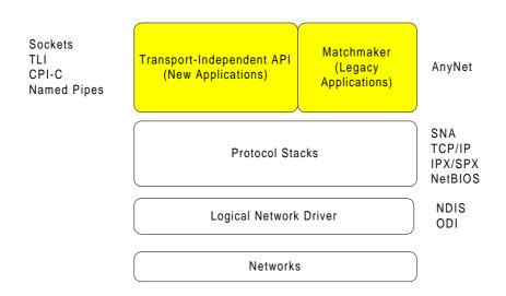
Figure 2. The bottom layers of the middleware.
