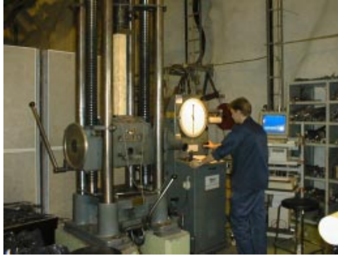
Figure 3.4. Heavy loading equipment is needed in compression tests.
