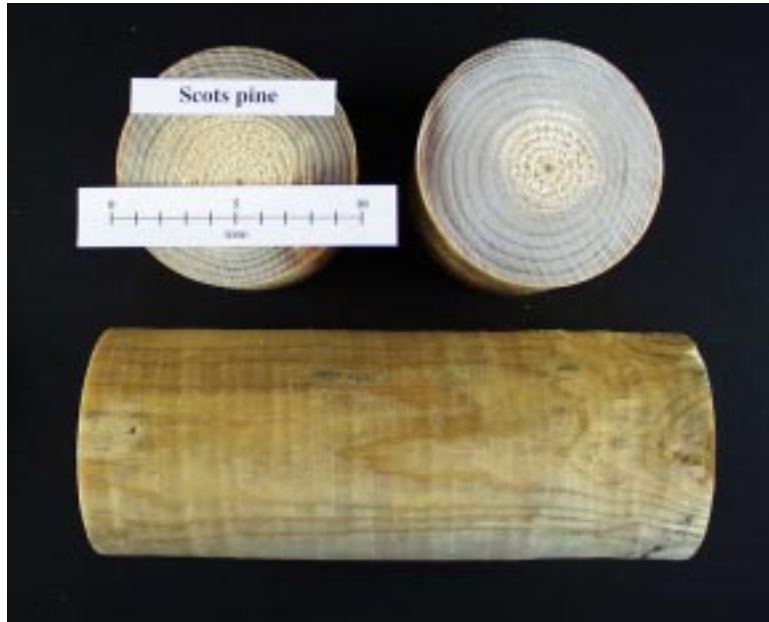
Figure 2.15. Scots pine after drying and treatment process.
