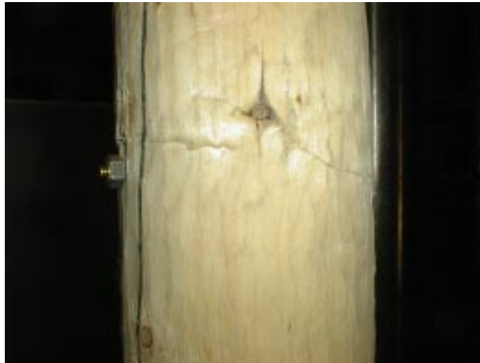
Figure 3.5. Local crushing in compression.
