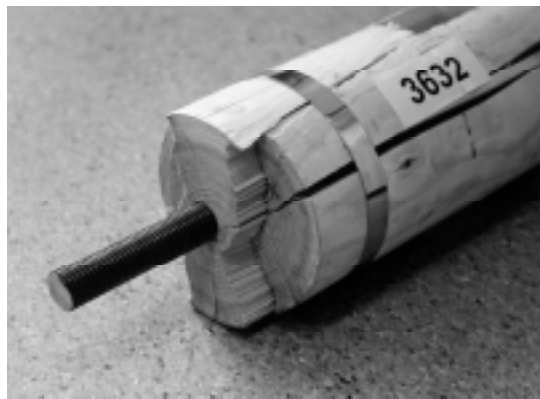
Figure 4.11. Typical shear failure.
