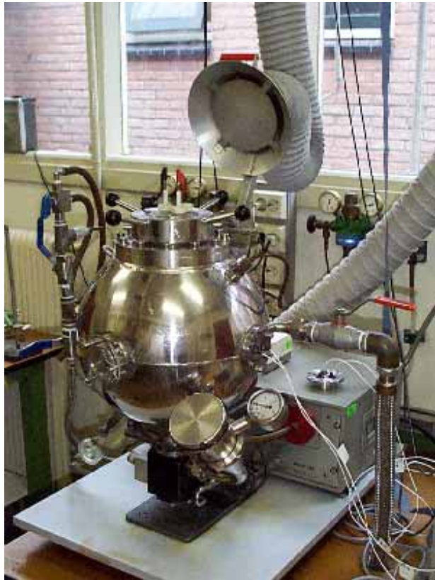
Figure 27. The standard 20 litre sphere for dust explosion research(TNO).
