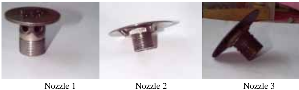
Figure 20. Dispersion nozzles designed and used by TNO.
