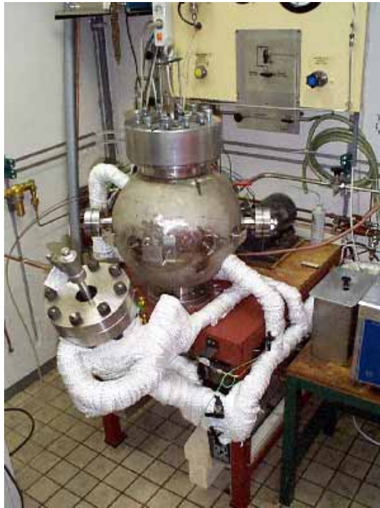
Figure 28. The strengthened 20-litre sphere for dust explosion research (insulation jacket removed)(TNO).
