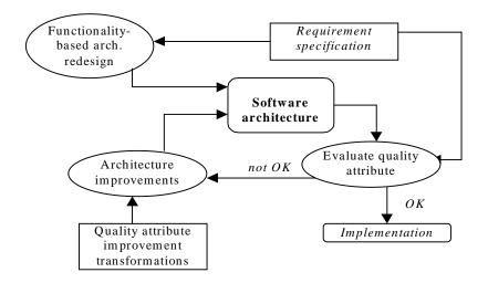
Figure 18. Reengineerining and architecture analysis by SBAR [9].
