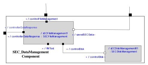
Figure 43. The structure diagram of the SEC\_DataManagement component.
