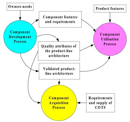
*Figure 1. Relationships between product line architecture, quality attributes and software components.*
