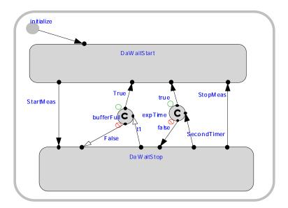
Figure 38. Statechart diagram of the SEC\_DataAcquisition concrete component.
