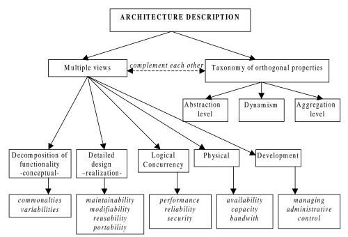
*Figure 8. Architecture description and the relevance to the analysis of quality attributes.*
