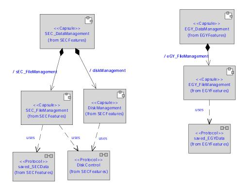
Figure 42. Specialization of the DataManagement in SECFeatures and EGYFeatures packages.
