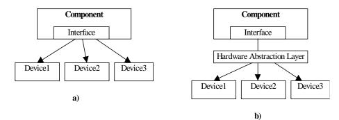
Figure 44. Decoupling of a software component from hardware.
