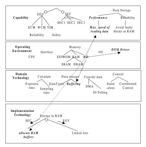
Figure 40. Adding new features in the problem domain together with the HD.
