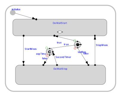
*Figure 39. Statechart diagram of the EGY\_DataAcquisition concrete component.*
