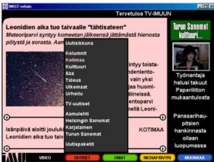
Figure 14. The TV-IMU is used with a TV remote control. The menu "Uutiset" is selected with the remote control red button. The channel "Kotimaa" is selected with the arrow keys. The browser is written in Java.
