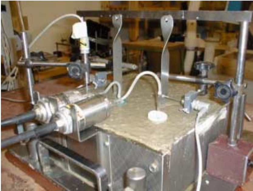
Figure 5.3. Picture of early age shrinkage test underway at VTT.
