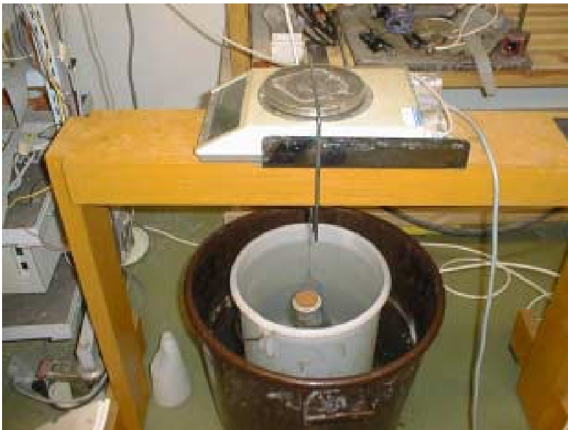
Figure 5.13. Side view of a chemical shrinkage test underway.
