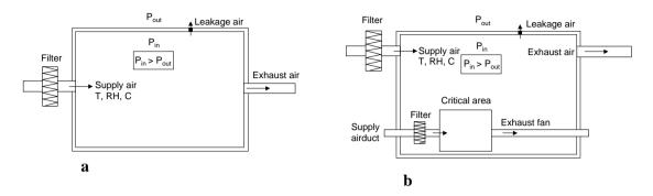
Figure 4. a) Mixing airflow and b) Unidirectional airflow (Lehtimäki, 1998).
