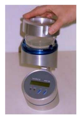
Figure 7. The MAS-100 air sampler is an impactor.
