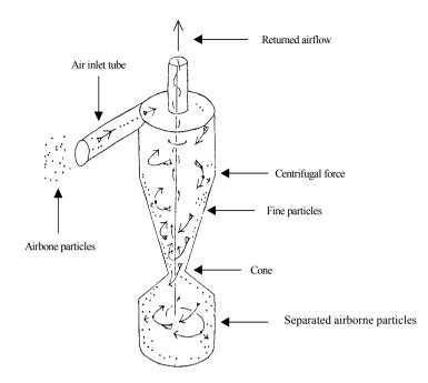
Figure 9. Centrifugal sampler (Cox, 1987).
