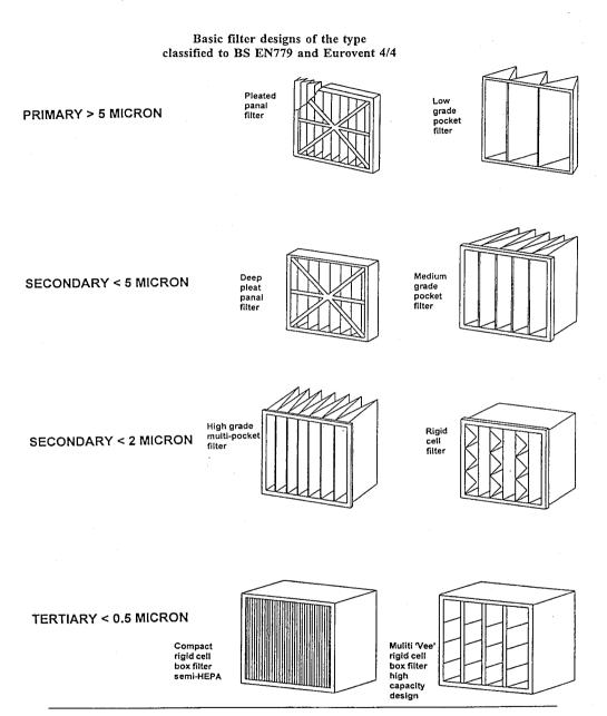
Figure 5. Basic filter designs of the type classified in BS EN779 and Eurovent 4/4 as well as EN1822 (Brown, 1996).
