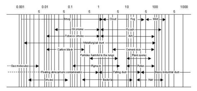
Figure 1. Particle size distribution (diameter as  $\mu m$ ) of some atmospheric contaminants (Brown, 1996).
