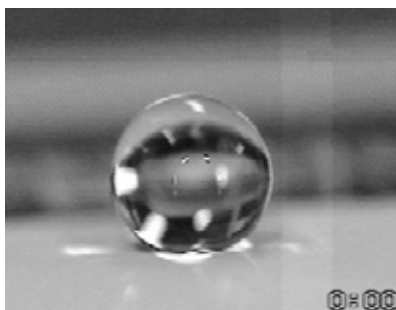
Figure 87. Droplet moving with the lowest achieved actuation voltage (124 V) 1 .
