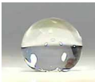
Figure 52. Water droplet (diameter 2 mm) on evaporated AKD surface.
