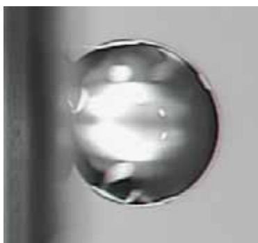
Figure 56. Water droplet (diameter ~1.6 mm) on vertically tilted O 2 plasma-etched Teflon ® AF.
