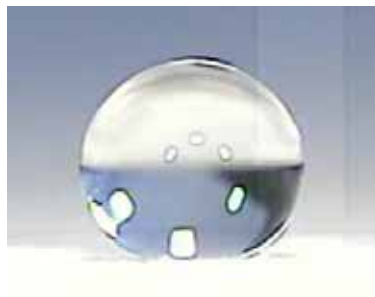
Figure 50. Water droplet (diameter 2 mm) on sprayed AKD surface.
