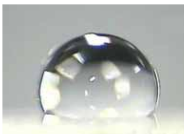
Figure 46. Water droplet (diameter 2 mm) on spin coated Teflon ® AF surface.
