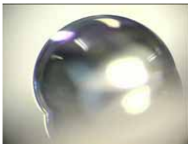
Figure 47. Water droplet (diameter 3.7 mm) on a tilted ICP fluoropolymer surface.
