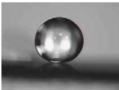
Figure 66. Droplet (diameter 1.4 mm) sliding on a tilted pillar FAS surface 1 .
