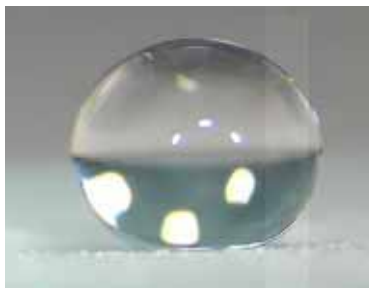
Figure 54. Water droplet (diameter 2 mm) on a sprayed Teflon ® AF surface.
